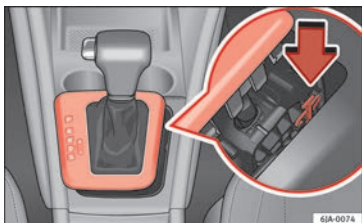
Fig. 135 Manual release of the selector lever.
