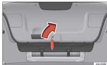
Fig. 134 Manual release of the rear lid
