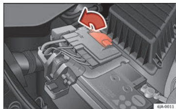
Fig. 115 Battery: Opening the cover.
