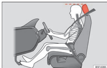
Fig. 2 Correct head restraint position for the driver.
