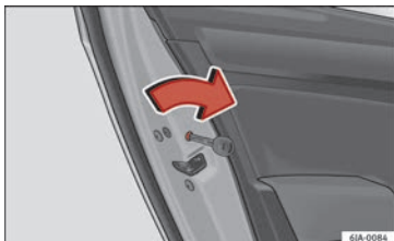
Fig. 40 Activating the childproof lock.
