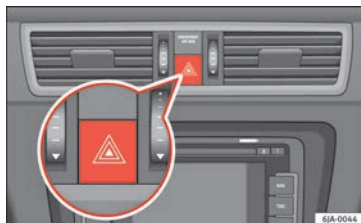
Fig. 49 Instrument panel: switch for hazard warning lights.
