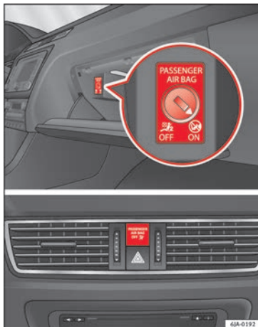
Fig. 18 Front passenger front airbag switch/warning lamp for disabling the front passenger airbag.
