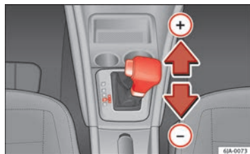
Fig. 93 Selector lever: Tiptronic.
