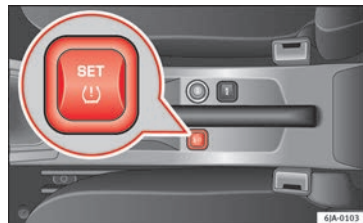
Fig. 120 Tyre pressure adjustment switch.
