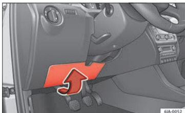
Fig. 138 Bottom of the dash panel: fuse cover.
