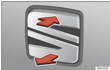
Fig. 42 Rear lid: opening from the outside.
