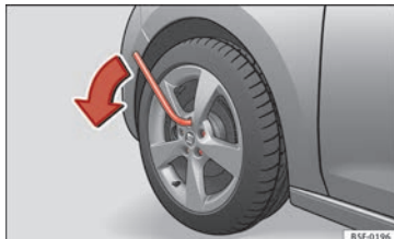
Fig. 124 Changing a wheel: loosen the wheel bolts.
