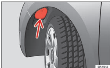
Fig. 146 Changing dipped beam headlight bulbs: wheel housing.
