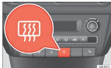
Fig. 53 Heated rear window switch.
