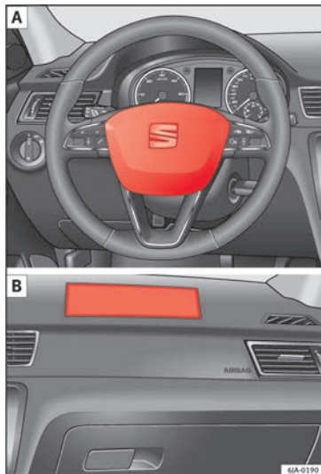
Fig. 12 Driver airbag in the steering wheel and front passenger airbag in the dash panel
