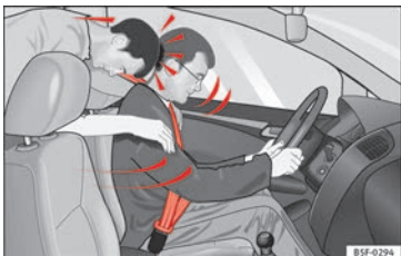
Fig. 8 The unbelted passenger in the rear seat is thrown forward violently, hitting the driver wearing a seat belt
