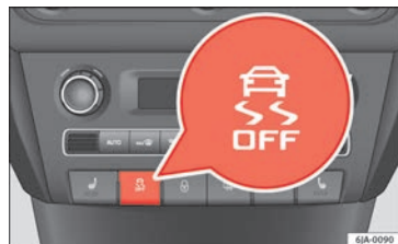
Fig. 95 ESC system: TCS switch.
