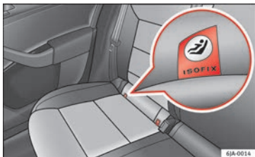
Fig. 21 ISOFIX securing rings.
