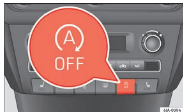
Fig. 98 Instrument panel: Start-Stop system button
