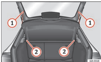
Fig. 82 Remove the shelf.
