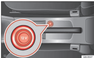
Fig. 71 Centre console: 12 V power socket.
