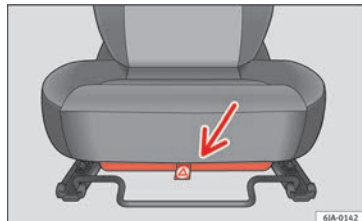
Fig. 66 Driver seat: storage compartment
