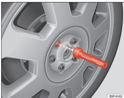
Fig. 172 Changing the wheel: Hexagonal socket in screwdriver handle to turn the wheel bolts
