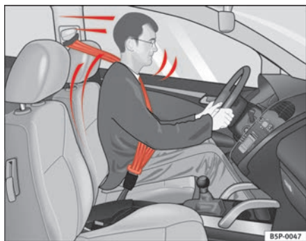
Fig. 11 Driver wearing the seat belt properly: is secured by the belt in sharp braking
