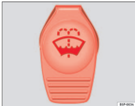
Fig. 164 In the engine compartment: Cap of windscreen washer fluid reservoir.
