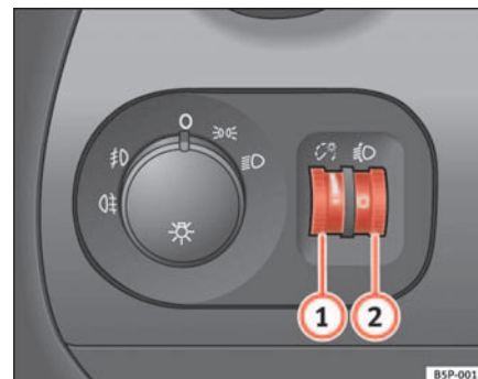
Fig. 75 Detail of the dash panel: Regulation for instrument and switch illumination and headlight range control
