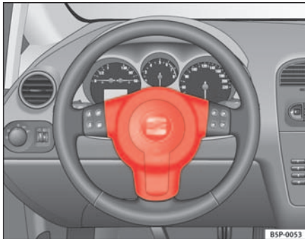
Fig. 18 Driver airbag located in steering wheel
