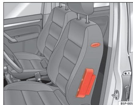
Fig. 22 Side airbag in driver seat
