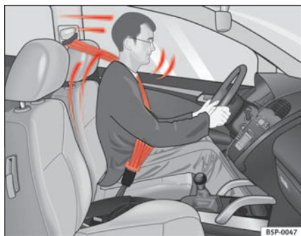
Fig. 11 Driver protected by the properly worn seat belt during a sudden braking manoeuvre.
