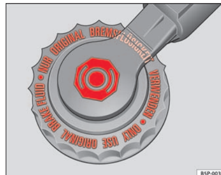
Fig. 168 In the engine compartment: Brake fluid reservoir cover
