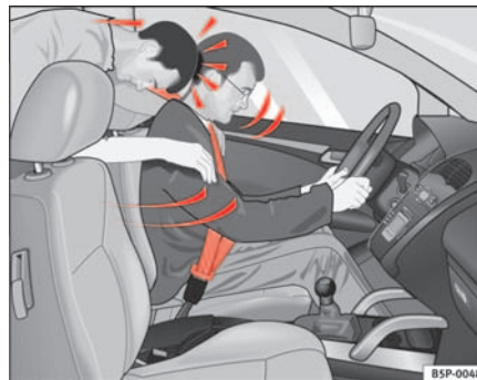
Fig. 10 The unbelted rear passenger is thrown forward violently, hitting the driver wearing a seat belt.
