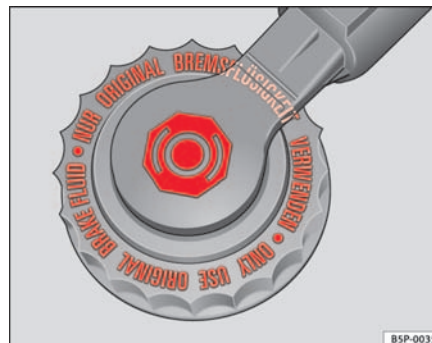
Fig. 161 In the engine compartment: Brake fluid reservoir cover
