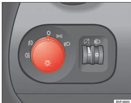
Fig. 74 Detail of the dash panel: Switch for lights, fog lights and rear fog light
