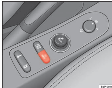
Fig. 48 Centre console: tyre monitor system button
