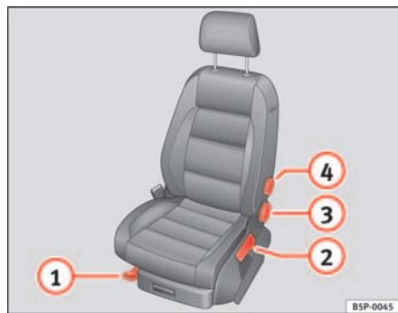
Fig. 94 Front left seat controls
