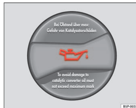
Fig. 155 In the engine compartment: Engine oil filler cap
