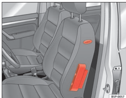
Fig. 22 Side airbag in driver seat
