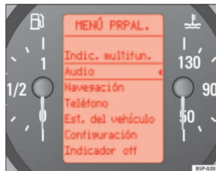
Fig. 44 Digital display on the instrument panel: Main menu
