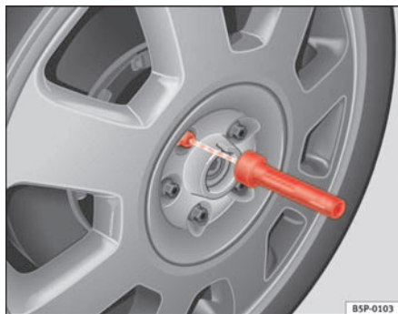
Fig. 169 Wheel change: Hexagon socket in screwdriver handle to turn the wheel bolts after they have been loosened
