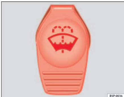
Fig. 157 In the engine compartment: Cap of windscreen washer fluid reservoir.
