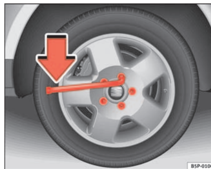
Fig. 166 Changing the wheel: Loosening the wheel bolts
