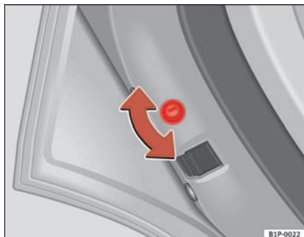
Fig. 61 Child safety lock on the left hand side door
