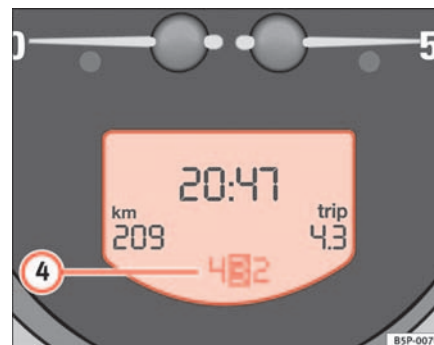
Fig. 37 Detail of instrument panel: Display with Tiptronic gear selection
