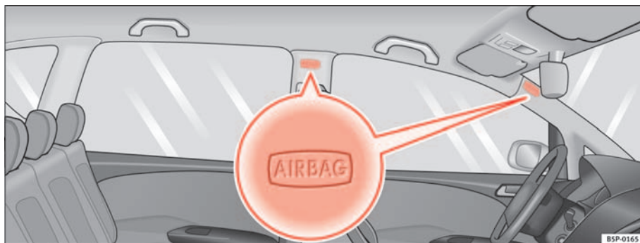
Fig. 24 Location of left curtain airbag
