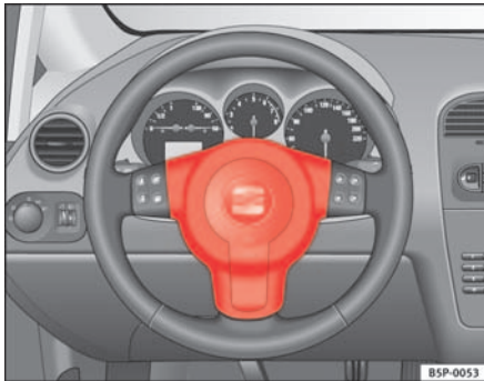
Fig. 18 Driver airbag located in steering wheel
