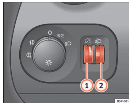
Fig. 76 Detail of the dash panel: Regulation for instrument and switch illumination and headlight range control
