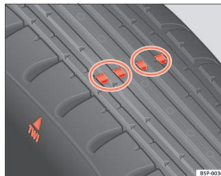
Fig. 162 Tyre tread wear indicators
