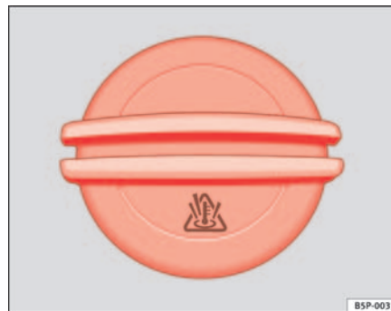
Fig. 156 In the engine compartment: Coolant expansion tank cap
