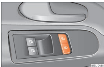
Fig. 69 On the driver's door: central locking buttons.
