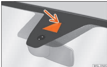
Fig. 140 On the windscreen: field of vision of the Lane Assist system.
