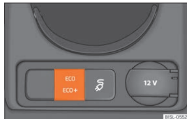
Fig. 138 In the lower part of the centre console: driving profile selection button.
