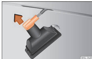
Fig. 55 Number plate light: remove the bulb holder.
