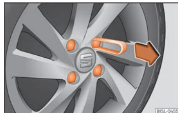
Fig. 31 Wheel: wheel nuts with caps.
