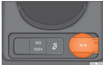
Fig. 105 Front centre console: 12-volt power outlet on the storage compartment and USB interface.
