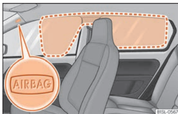
Fig. 19 Location and deployment area of the head-protection airbag.
