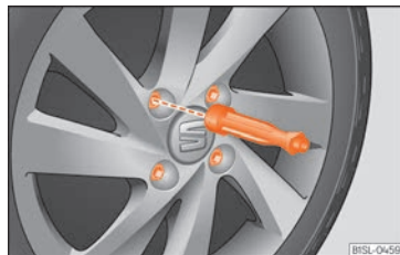
Fig. 37 Wheel change: loosen wheel nuts using the socket in the handle of the screwdriver.
