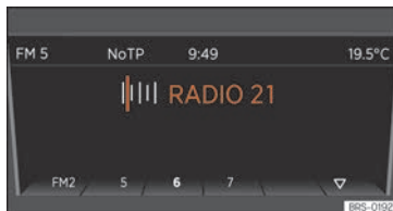
Fig. 114 Changing the stations with the arrow buttons is only possible for saved stations.
