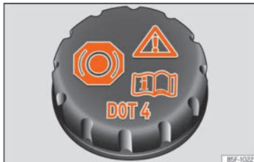
Fig. 165 Engine compartment: brake fluid reservoir cap.
