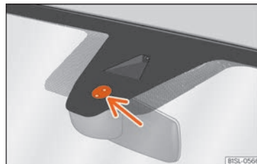
Fig. 86 Rain sensor sensitive surface
