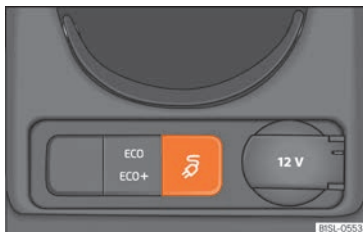
Fig. 152 At the bottom of the centre console: charging mode button.
