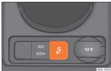
Fig. 155 At the bottom of the centre console: charging mode button.
