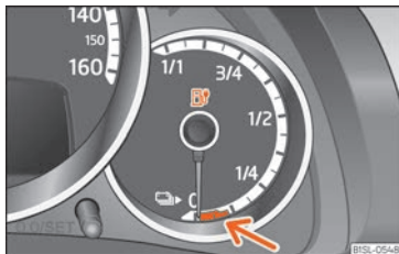
Fig. 148 On the instrument panel: indicator of the high-voltage battery charge level with the reserve area marked in red (arrow).
