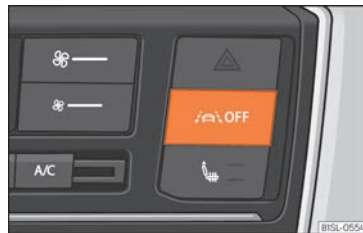
Fig. 141 In the centre console: button to connect the lane assist system
