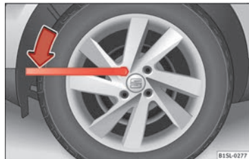
Fig. 127 Changing a wheel: Slacken the wheel bolts.
