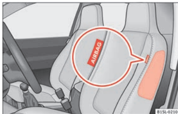
Fig. 14 On the side of the front seat: location of the side airbag
