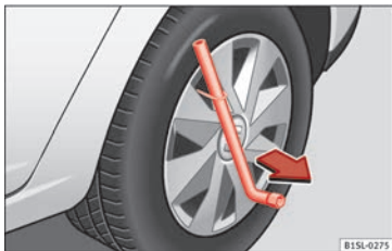
Fig. 125 Removing the full hubcap
