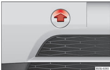
Fig. 135 On the right-hand side of the front bumper: Remove the cover.
