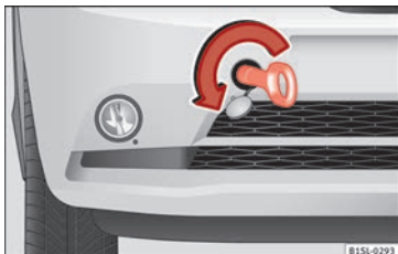
Fig. 136 On the right-hand side of the front bumper: Screw in the towline anchorage.
