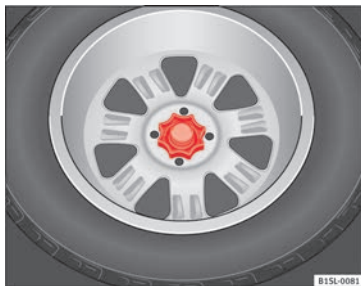
Fig. 118 In the luggage compartment: hand controlled wheel for securing the spare wheel
