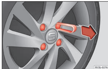
Fig. 126 Removing the wheel bolt caps
