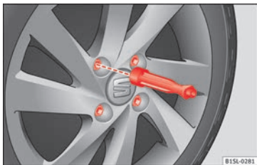
Fig. 131 Changing a wheel: loosen wheel bolts with the socket at the end of the wheel brace
