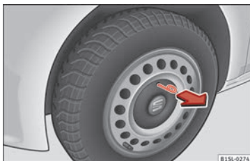
Fig. 124 Remove the hubcap of the steel wheel trim
