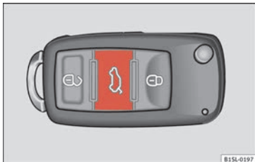
Fig. 37 On the vehicle key: button to unlock and open the boot hatch.
