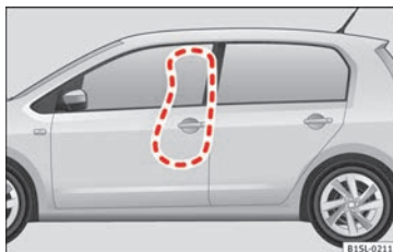
Fig. 15 On the left side of the vehicle: deployment area of side airbag
