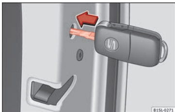
Fig. 139 Emergency locking of the vehicle using the vehicle key
