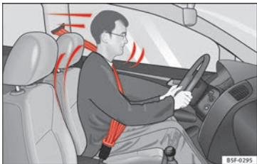
Fig. 7 Drivers with properly worn seat belts will not be thrown forward in the event of sudden braking
