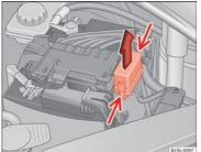
Fig. 151 In the engine compartment: fuse box cover
