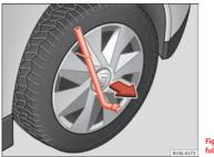
Fig. 142 Removing the full hubcap
