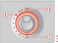
Fig. 26 In the interior roof: turn the knob to open and close
