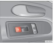
Fig. 24 In the driver door: electric windows button
