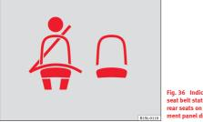
Fig. 36 Indication of seat belt status in the rear seats on the instrument panel display
