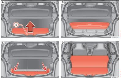
Fig. 69 A: Open the luggage compartment variable floor. B: raised luggage compartment variable floor.
