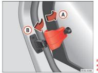
Fig. 25 Lever to open and close the rear window
