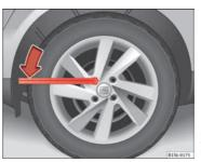
Fig. 144 Changing a wheel: Slacken the wheel bolts.
