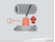
Fig. 161 Side turn signal: Changing the bulbs
