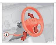
Fig. 33 Mechanical steering wheel adjustment Adjust the steering wheel before your trip and only when the vehicle is stationary.
