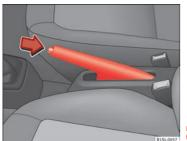
Fig. 93 Between the front seats: Handbrake
