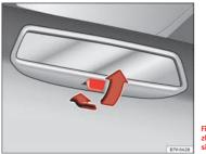
Fig. 64 Manual anti-dazzle function for rear vision mirror
