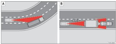
Fig. 102 A: Vehicle on a bend. B: Motorcyclist driving ahead out of range of the laser sensor
