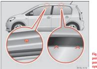
Fig. 72 Attachment points for the basic support and the roof carrier system
