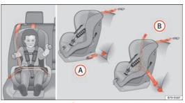
Fig. 52 On the rear seats: figure () shows the basic child restraint system mounting using lower retaining rings and the upper retaining strap figure () shows the child restraint system mounting using the vehicle seat bet
