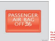
Fig. 46 Control lamp for disabling the front passenger front airbag on the dash panel
