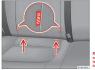
Fig. 53 On the vehicle seat: Identification variants of the anchor points for the child seats Each seat of the rear seat bench has **two** retainers named lower anchor points.
