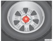
Fig. 126 In the luggage compartment: hand controlled wheel for securing the spare wheel
