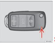
Fig. 14 Control lamp on the vehicle key
