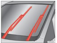
Fig. 62 Wipers in service position
