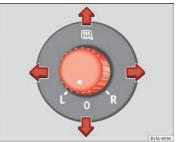
Fig. 66 In the driver door: rotary control for the exterior electric mirrors
