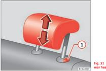
Fig. 31 Adjusting the rear head restraints
