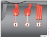
Fig. 87 Pedals in vehicles with a manual gearbox: (1) accelerator; (2) brake; (3) clutch
