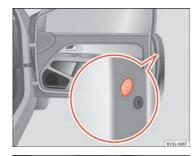
Fig. 136 To the front of the passenger side door: Emergency lock, hidden by a rubber cap
