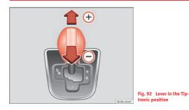
With Tiptronic, the gears can be changed up or down manually with the automatic gearbox. When you change to the Tiptronic programme, the vehicle remains in the currently selected gear. This is possible as long as the system is not changing gear automatically due to a traffic situation.
