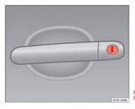
Fig. 135 Driver side door handle with lock cylinder
