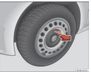
Fig. 141 Remove the hubcap of the steel wheel trim
