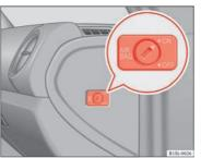
Fig. 49 On front passenger side: key switch for disabling and enabling the front passenger front airbag
