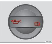
Fig. 115 In the engine compartment: Engine oil filler cap
