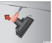
Fig. 159 Number plate light: Remove the lamp holder
