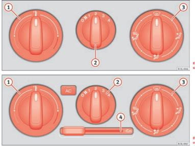
Fig. 105 In the centre console: Heating and ventilation system rotary control
