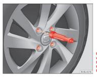
Fig. 148 Changing a wheel: loosen wheel bolts with the socket at the end of the wheel brace
