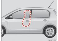
Fig. 51 On the left side of the vehicle: deployment area of side airbag
