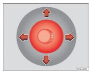
Fig. 65 In the front doors: button to adjust the mechanical exterior rear vision mirror
