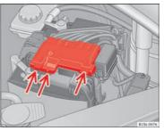
Fig. 118 In the engine compartment: Remove the cover from the vehicle's battery
