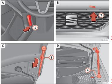
Fig. 112 A: Release lever in the footwell on the driver side B: Release lever on the bonnet
