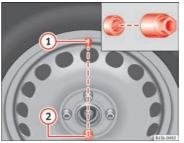
Fig. 145 Changing a wheel: Tyre valve ① and position of anti-theft wheel locking bolt ②
