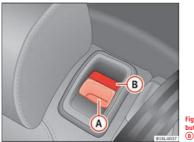
Fig. 67 Rear seat: unlock button (A); red marking
