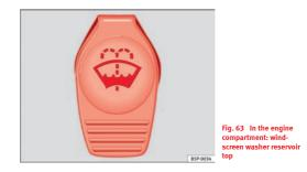
Check the water level in the windscreen washer reservoir regularly and top up as required.
