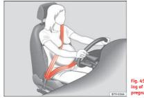
Fig. 45 Correct positioning of seat belts during pregnancy
