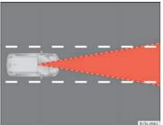
Fig. 100 Laser sensor detection area
