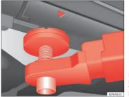
Fig. 131 Rear jacking points for raising vehicle with lifting platform or jack
