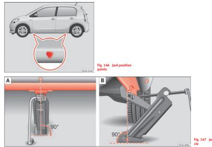
Fig. 147 jack mounted on the left rear part of the vehi-
