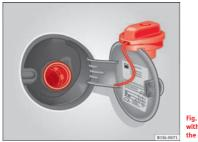
Fig. 110 Open tank flap with tank cap attached to the holder
