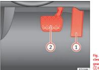
Fig. 88 Pedals in vehicles with an automatic qearbox: (1) accelerator; (2) brake
