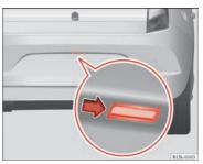
Fig. 158 On the rear bumper: Remove number plate light
