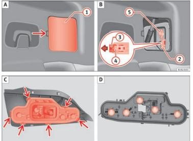
Fig. 156 On the side of the luggage compartment: A: Remove the cover, B: Removing the tail light units
