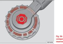
Fig. 94 In the engine compartment: brake fluid reservoir, lid
