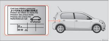
The correct tyre pressures for tyres fitted at the factory is shown on a label and is valid for summer and winter tyres. This label  $\Rightarrow$  Fig. 124 is either in the driver door strut or inside the fuel cap.
