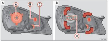
Fig. 153 In the engine compartment: Rearview of the front left headlight with rubber cover: (a) dipped beam and main beam headlights, (b) side lights and daytime driving lights and (c) turn signal
