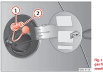
Fig. 111 Tank flap open: gas filler mouth (1), filler mouth retainer (2)
