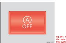
Fig. 104 At the top of the centre console: Start-Stop system button
