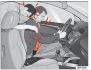
Fig. 40 The unbelted rear passenger is thrown forward violently, hitting the driver wearing a seat belt
