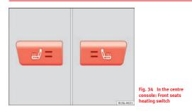
The front seat cushions can be heated electrically when the ignition is switched on.
