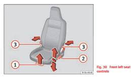
The controls are mirrored for the front right-hand seat.
