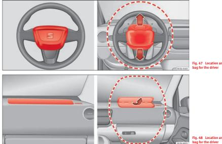
Fig. 47 Location and deployment area of the front airbag for the driver
