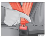
Fig. 42 Insert the latch plate into the buckle
