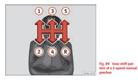
The position of each of the gears is shown on the gear stick  $\Rightarrow$  Fig. 89.
