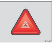
Fig. 133 Dash panel: Button to switch on and off the hazard warning lights system
