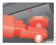
Fig. 130 Front jacking points for raising vehicle with lifting platform or jack
