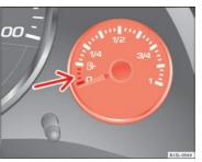
Fig. 108 On the instrument panel: fuel gauge for petrol
