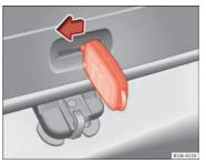
Fig. 138 From the luggage compartment: Manually unlocking the rear lid
