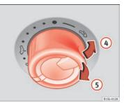
Fig. 27 In the interior roof: turn the knob to raise and to close the sunroof
