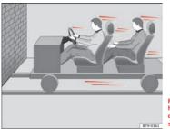
Fig. 37 Vehicle about to hit a wall: the vehicle occupants are not wearing seat belts
