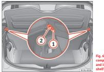
Fig. 68 In the luggage compartment: removing and installing the rear shelf
