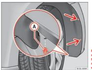
Fig. 154 In the front right wheel arch: Remove the retaining screws (arrows) and take out the expansive rivet (A).
