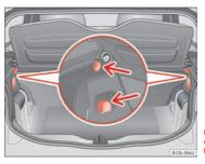
Fig. 71 In the luggage compartment: retaining hooks
