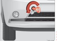
Fig. 165 On the righthand side of the front bumper: Screw in the towline anchorage
