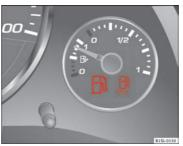
Fig. 109 On the instrument panel: fuel gauge for petrol and natural gas.
