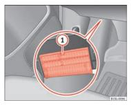
Fig. 150 Below the driver side dash panel: fuse box cover
