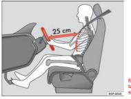
Fig. 28 The proper distance between driver and steering wheel
