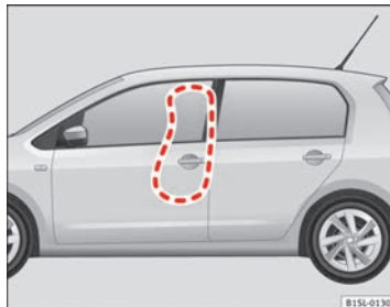
Fig. 51 On the left side of the vehicle: deployment area of side airbag
