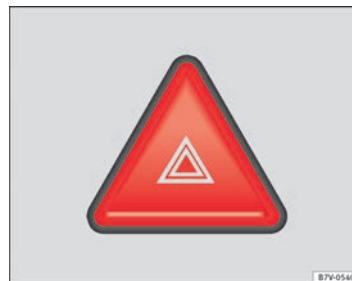
Fig. 130 Dash panel: Button to switch on and off the hazard warning lights system
