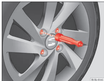
Fig. 145 Changing the wheel: loosen wheel bolts with the socket at the end of the wheel brace
