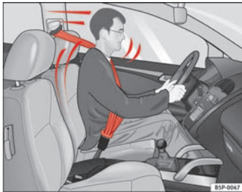
Fig. 41 Drivers with properly worn seat belts will not be thrown forward in the event of sudden braking
