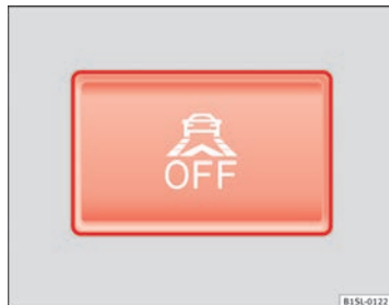
Fig. 98 In the lower part of the centre console: Button for the City Safety Assist function
