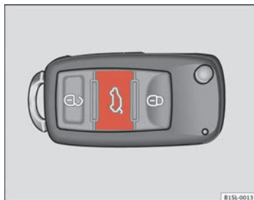
Fig. 22 On the vehicle key: Button to unlock and open the rear lid
