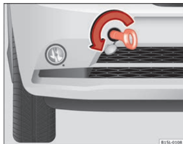
Fig. 162 On the right-hand side of the front bumper: Screw in the towing ring
