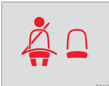
Fig. 36 Indication of seat belt status in the rear seats on the instrument panel display
