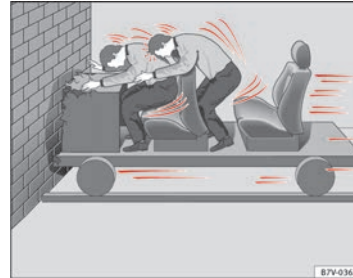
Fig. 38 The vehicle hits the wall: the occupants are not wearing seat belts
