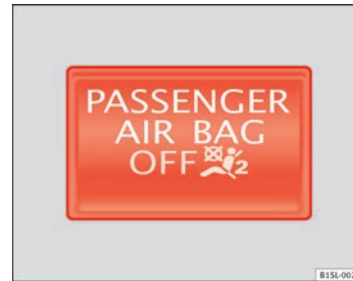
Fig. 46 Control lamp for disabling the front passenger airbag on the dash panel
