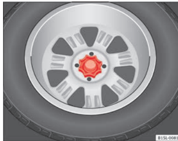
Fig. 123 In the luggage compartment: hand controlled wheel for securing the spare wheel
