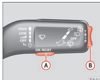
Fig. 11 Windscreen wiper lever: button (A) to confirm the options and rocker switch (B) to change the options
