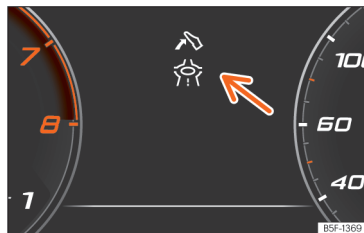
Fig. 102 Eco-efficient driving assistance indication [schematic representation].
