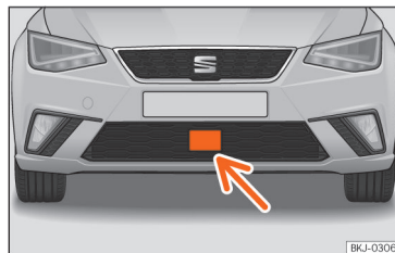
Fig. 94 On the front bumper: radar sensor.
