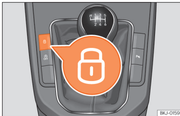
Fig. 50 Centre console: central locking switch.
