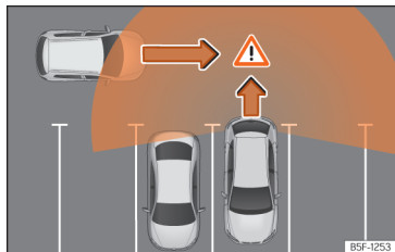
Fig. 124 Diagram of the parking assistant: detected area around the vehicle that is driving off.
