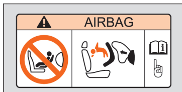
Fig. 33 Airbag sticker: on the passenger side sunshade blind.
