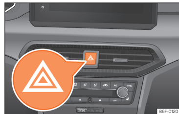
Fig. 41 Dashboard: switch for hazard warning lights.
