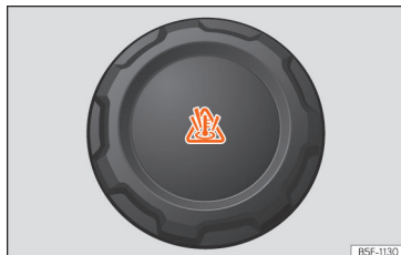
Fig. 173 Front compartment: coolant expansion tank cap.
