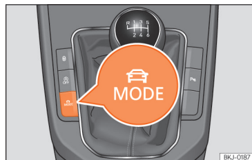
Fig. 91 Next to the gearbox lever: MODE button.
