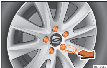
Fig. 187 Wheel: wheel nuts with caps.
