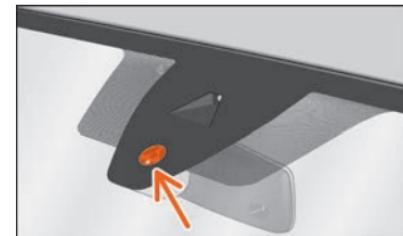
**Fig. 74** Sensitive surface of the rain sensor.
