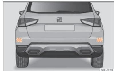
**Fig. 95** Rear view of the vehicle: radar sensor areas.
