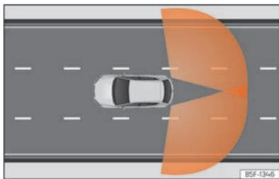
**Fig. 96** Sensor detection zones.
