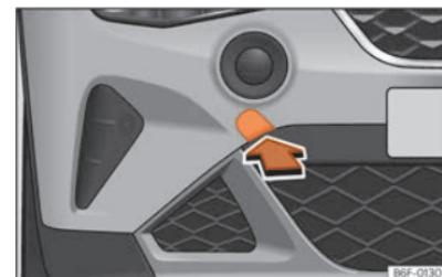
Fig. 164 Front bumper on right: remove the lid.
