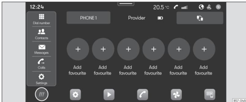
You can use the telephone interface to connect your mobile to the infotainment system and operate phone functions through it. The sound is played through the vehicle's speakers.
