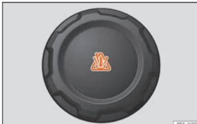
**Fig. 181** Front compartment: coolant expansion tank cap.
