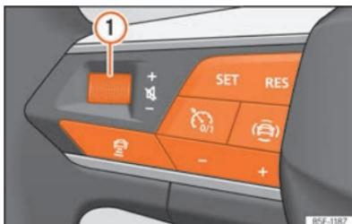
Fig. 58 Controls on the steering wheel.
