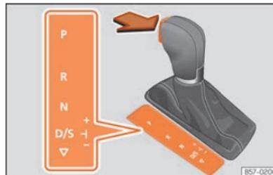
**Fig. 85** Selector lever lock.
