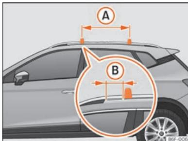
**Fig. 148** Attachment points for the crossbars for the roof carrier
