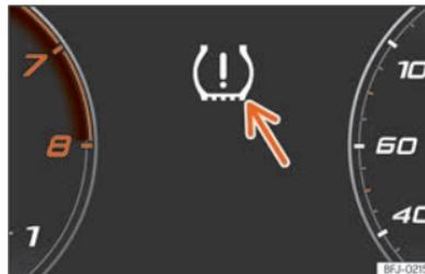
**Fig. 200** Instrument cluster: warning of loss of tyre pressure.
