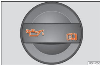
**Fig. 187** Oil filler cap cover in the engine compartment.
