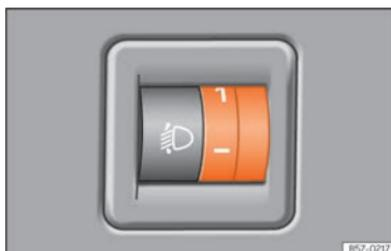
**Fig. 70** Next to the steering wheel: headlight range control regulator.
