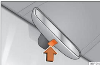
**Fig. 75** Manual anti-dazzle function for interior mirror
