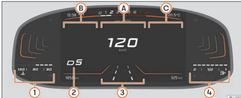
**Upper zone:** Time, selected drive profile, rev counter, outside temperature. **Lower zone:** total km (miles) or speed set with the cruise control or ACC, range.
