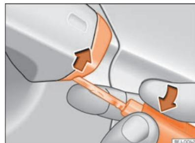
**Fig. 52** Driver's door handle: pry the cover open.
