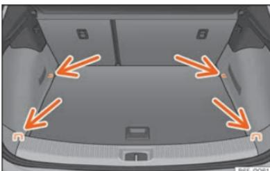
**Fig. 147** Location of fastening rings in luggage compartment.
