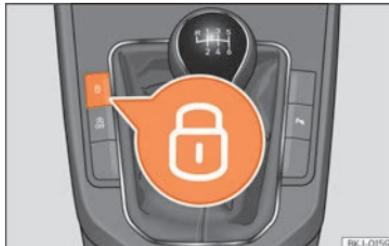
**Fig. 50** Centre console: central locking switch.
