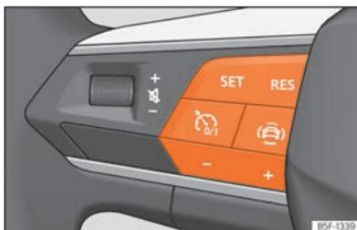
**Fig. 98** On the multifunction steering wheel: cruise control operation buttons.
