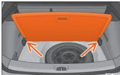
**Fig. 146** Variable boot floor: tilted position.
