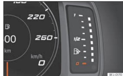
Fig. 4 SEAT Digital Cockpit instrument cluster: fuel gauge.
