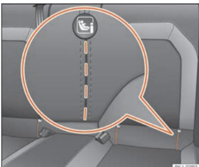
**Fig. 35** Rear seat: slots pre-punched to access the ISOFIX / iSize securing rings.
