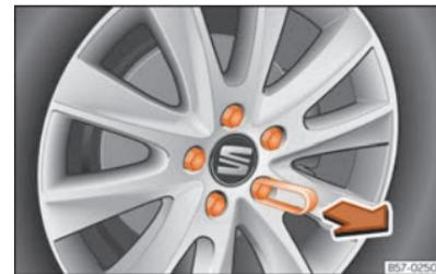
**Fig. 194** Wheel: wheel nuts with caps.
