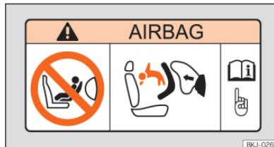
Fig. 33 Airbag sticker: on the passenger side sunshade blind.
