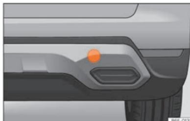
**Fig. 166** Rear bumper on right: remove the lid.
