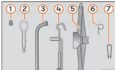
**Fig. 157** Underneath the floor panel of the luggage compartment: on-board tools.
