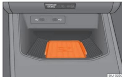
**Fig. 142** On the centre console: pad for the mobile phone connection.
