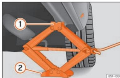
Fig. 199 Crossbar: mounting the jack on the vehicle.
