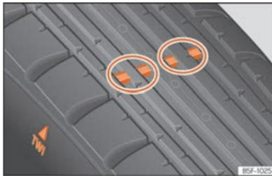
Fig. 190 Tyre profile: tread wear indicators.
