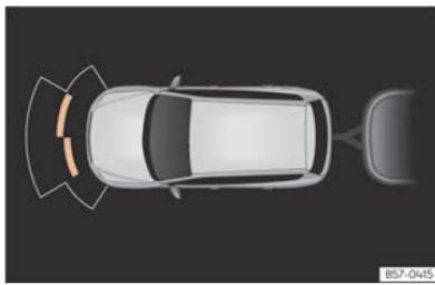
**Fig. 119** Parking assist display on the screen with trailer attached.
