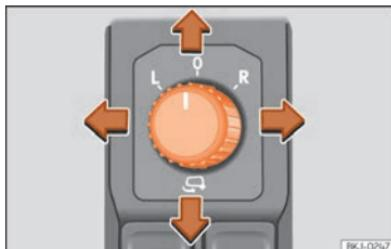
**Fig. 76** Driver's door detail: exterior mirror control.
