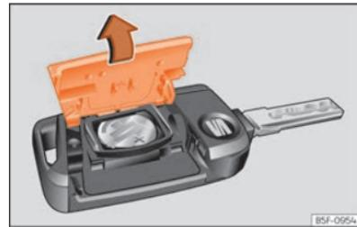
**Fig. 45** Vehicle key: opening the battery compartment.
