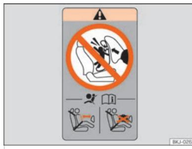
Fig. 34 Airbag sticker: at the bottom of the passenger door frame.
