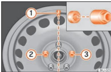
**Fig. 197** Tyre change: tyre valve **1** and the correct position for the anti-theft wheel locking bolt **2** or **3**.
