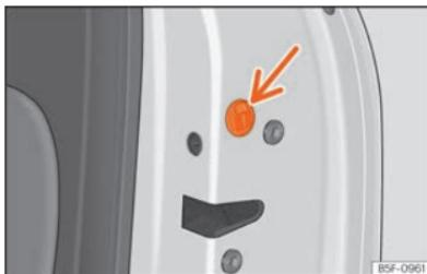
**Fig. 53** Locking the door manually.
