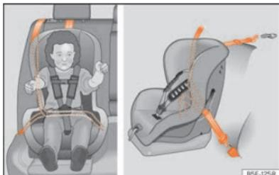
Fig. 39 On rear seats: installing a child seat.
