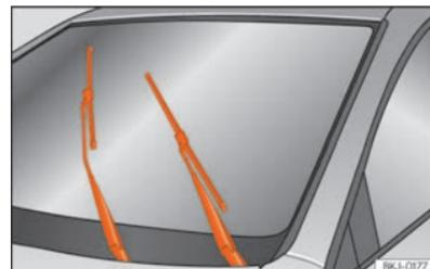
**Fig. 158** Wipers in service position.
