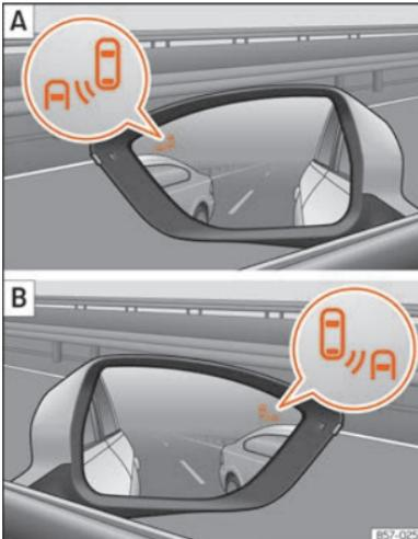
**Fig. 114** Control lamp of the lane departure warning.
