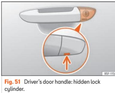
**Fig. 51** Driver's door handle: hidden lock cylinder.
