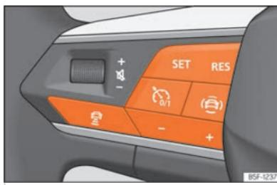
**Fig. 102** On the multifunction steering wheel: buttons for operating the ACC.
