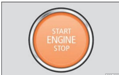
**Fig. 81** In the lower part of the centre console: start button.
