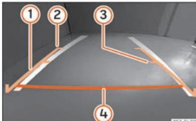
**Fig. 129** Infotainment system display: guidance lines.
