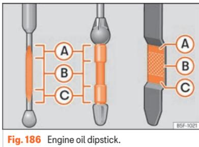
**Fig. 186** Engine oil dipstick.
