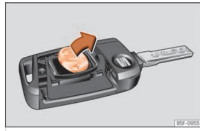
**Fig. 46** Vehicle key: removing the battery.
