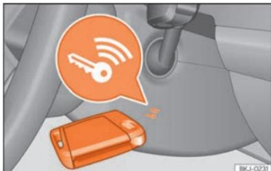
**Fig. 82** On the right of the steering column: emergency start.
