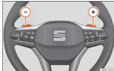
Fig. 87 Steering wheel: automatic gearbox levers
