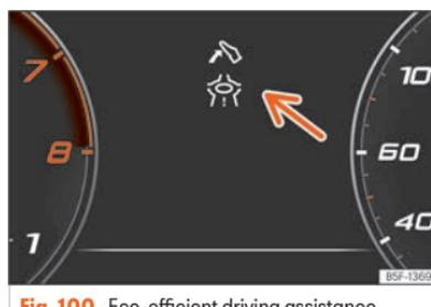
**Fig. 100** Eco-efficient driving assistance indication [schematic representation].
