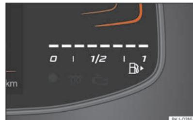
Fig. 3 Basic instrument cluster: fuel gauge.
