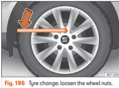
**Fig. 196** Tyre change: loosen the wheel nuts.
