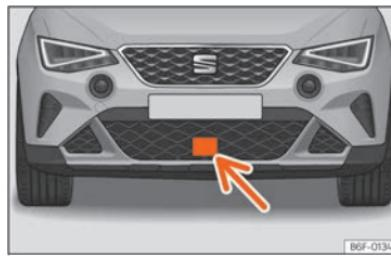
**Fig. 92** On the front bumper: radar sensor.
