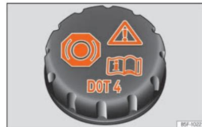
Fig. 182 Engine compartment: brake fluid reservoir cap.
