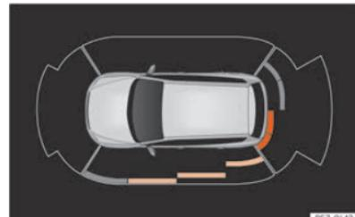
**Fig. 121** Parking aid view on the Infotainment system display.
