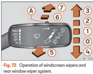
Fig. 72 Operation of windscreen wipers and rear window wiper system.
