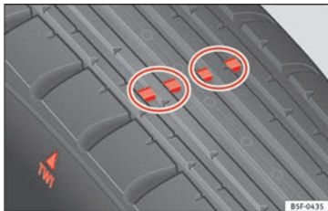
Fig. 251 Tyre tread: tread wear indicators
