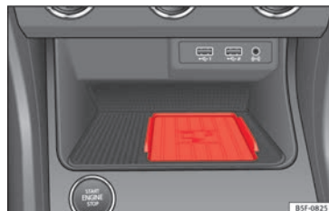
Fig. 131 Centre console: Connectivity Box.
