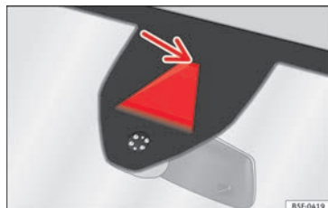
Fig. 216 In the windscreen: field of vision of the Lane Assist system camera.
