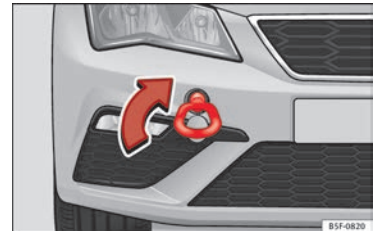
Fig. 77 Right side of the front bumper: towline anchorage screwed in.
