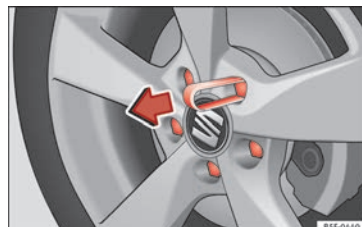
Fig. 72 Wheel: wheel bolts with caps.
