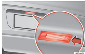
Fig. 118 In the rear bumper: number plate light.
