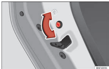
Fig. 139 Childproof lock on the left hand side door.
