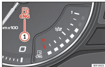
Fig. 126 Instrument panel: Natural gas gauge
