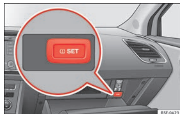
Fig. 254 Glove compartment: tyre control switch.
