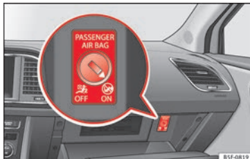
Fig. 22 Front passenger front airbag switch.
