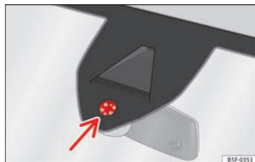
Fig. 148 Rain sensor sensitive surface
