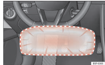
Fig. 25 On the driver side: radius of action of the knee airbag.
