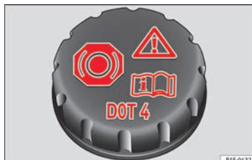
Fig. 64 Engine compartment: brake fluid reservoir cap.
