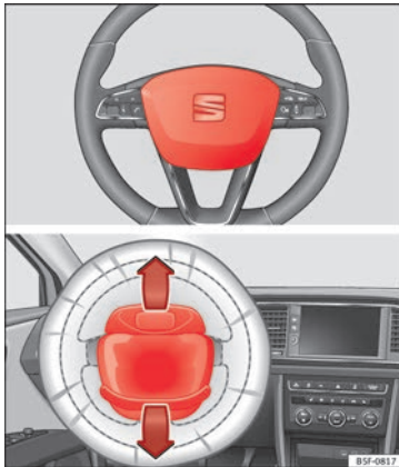
Fig. 20 Driver airbag located in steering wheel.
