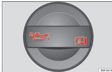
Fig. 62 In the engine compartment: Engine oil filler cap.
