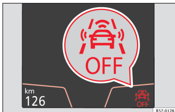
Fig. 206 On the instrument panel display: Front Assist switched off message.
