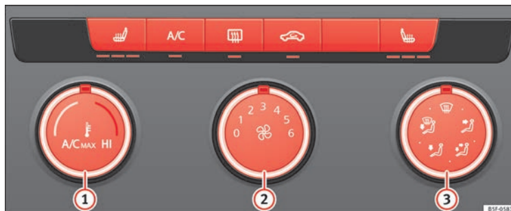
Fig. 58 In the centre console: Manual air conditioning controls.
