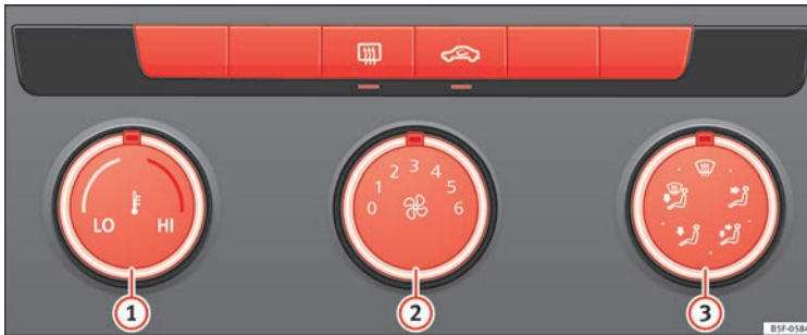
Fig. 59 In the centre console: heating system and fresh air controls.
