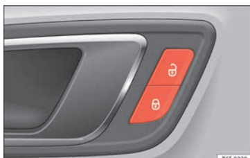
Fig. 2 Driver door: central locking switch.
