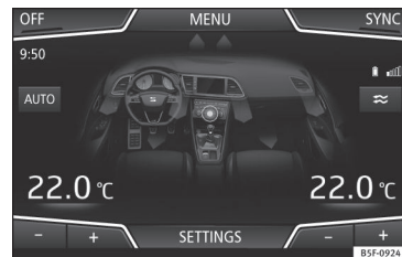
Fig. 189 Easy Connect screen: air conditioner menu.
