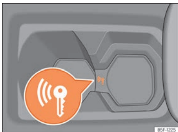
Fig. 116 On the centre console: emergency start.
