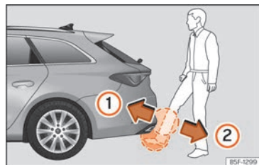
Fig. 81 Rear lid with sensor-controlled opening (Easy Open).
