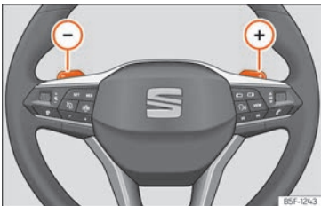
Fig. 120 Steering wheel: automatic gearbox levers
