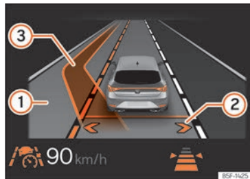
Fig. 142 On the instrument cluster screen: lane change assist display (schematic representation).
