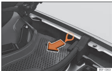
Fig. 62 Between the left wing panel and the engine bonnet hinge: Charging connector manual release mechanism puller.
