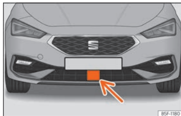
Fig. 123 On the front bumper: radar sensor.
