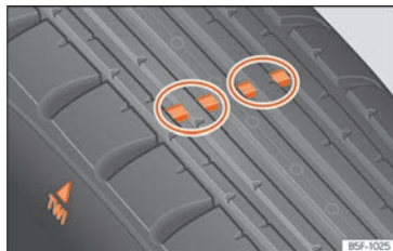
Fig. 234 Tyre profile: tread wear indicators.
