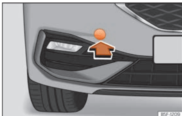
Fig. 212 Front bumper on right: remove the lid.
