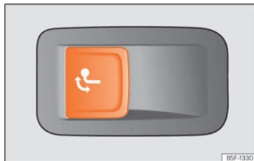
Fig. 198 Left side of the luggage compartment: button to unlock the tow hitch.
