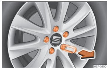
Fig. 239 Wheel: wheel bolts with caps.
