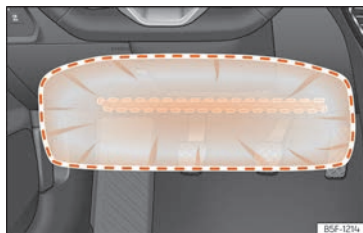
Fig. 40 On the driver side: action radius of airbag for knees.
