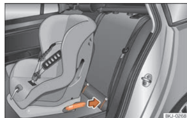
Fig. 46 Rear seats: fitting a child seat with the ISOFIX system.
