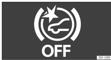
Fig. 138 On the screen of the instrument panel Front Assist switched off message.
