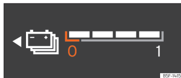
Fig. 9 Digital instrument cluster: battery level indicator.
