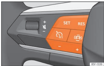
Fig. 130 On the multifunction steering wheel: buttons to control the speed limiter.
