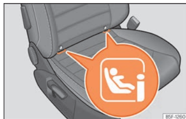
Fig. 45 Front passenger seat: location of the i-Size fastening rings.
