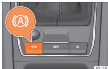
Fig. 148 In the lower part of the centre console: Auto Hold function button.
