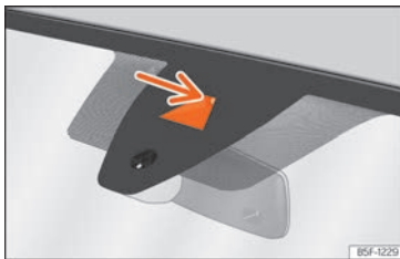
Fig. 125 On the windscreen: field of vision of the Lane Assist system camera.
