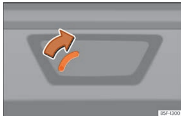
Fig. 83 Luggage compartment: manual release (Leon Sportstourer).
