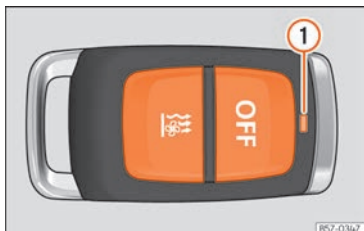
Fig. 114 Independent heating: radiofrequency remote control key
