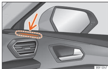
Fig. 144 Control lamp of the lane departure warning.
