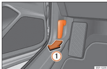
Fig. 219 Release lever in the driver's footwell area.
