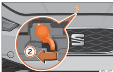
Fig. 200 Lever under the bonnet.
