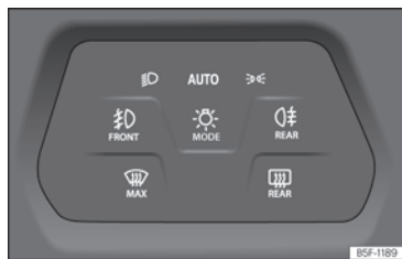
Fig. 90 Dash panel: lights control.
