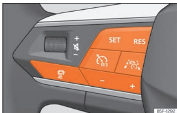
Fig. 173 Left side of the multifunction steering wheel: buttons for operating Travel Assist.
