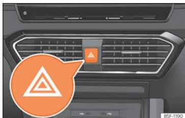
Fig. 92 Dash panel: hazard warning lights switch
