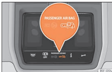
Fig. 18 On the roof console: control lamp for the deactivation of the front passenger front airbag.
