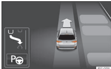
Fig. 184 On the instrument panel display: view of the parking assist system with reduced view.
