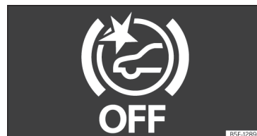
Fig. 160 On the instrument panel display: Front Assist deactivated indication.
