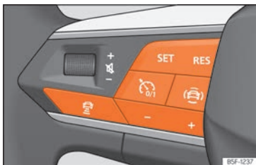
Fig. 165 On the multifunction steering wheel: buttons to operate the ACC
