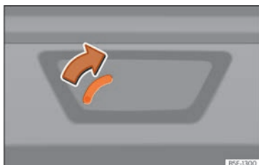
Fig. 86 Detail of the luggage compartment: emergency unlocking (Leon Sportstourer).
