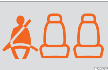
Fig. 7 Instrument panel: left rear seat occupied and corresponding seat belt fastened display.
