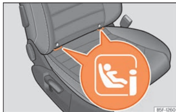
Fig. 28 Front passenger seat: ISOFIX/i-Size securing rings.
