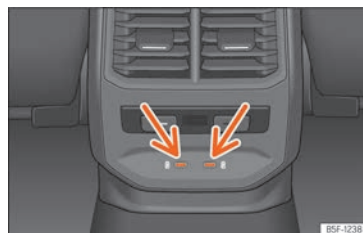
Fig. 146 Rear part of the centre console: USB connectors with power outlet function.
