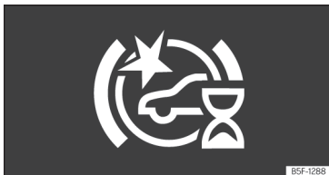
Fig. 159 On the instrument panel display: initial system self-calibration indication.
