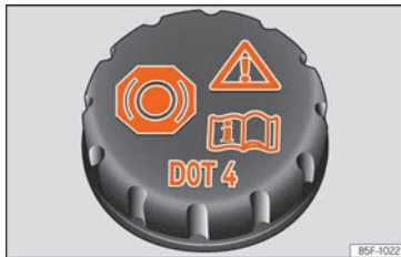
Fig. 206 Engine compartment: brake fluid reservoir cap.
