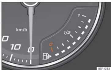
Fig. 58 Analogue instrument panel: fuel gauge
