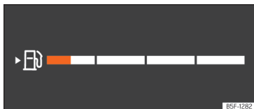
Fig. 59 Digital instrument panel: fuel level indicator located in different positions depending on the view.
