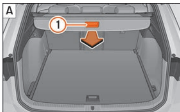
Fig. 113 In the luggage compartment: removing the shelf.
