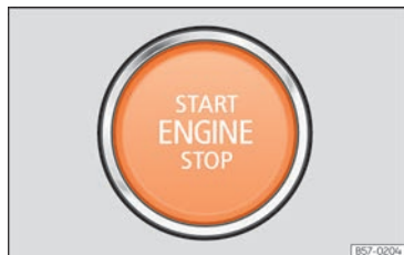
Fig. 147 In the lower part of the centre console: start button.
