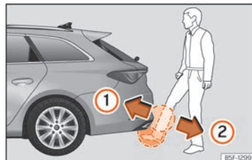
Fig. 84 Rear lid with sensor-controlled opening (Easy Open).
