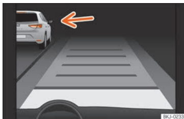
Fig. 166 On the instrument panel display: ACC active, vehicle detected in an outer lane.
