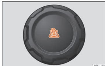
Fig. 205 Engine compartment: coolant expansion tank cap.
