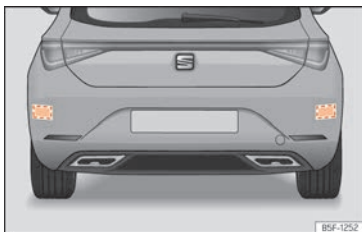
Fig. 176 Rear view of the vehicle: radar sensor zones.
