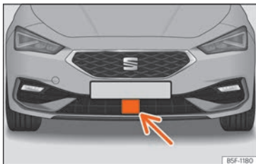
Fig. 161 On the front bumper: radar sensors.
