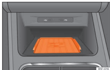
Fig. 144 In the centre console: pad for the mobile phone connection.
