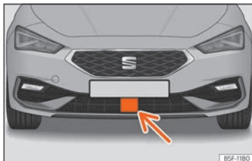
Fig. 164 On the front bumper: radar sensors.
