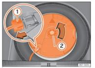
**Fig. 329** In the luggage compartment: remove the subwoofer.
