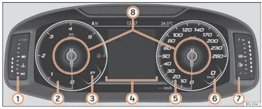
**Fig. 75** SEAT Digital Cockpit on the instrument panel (classic view).
