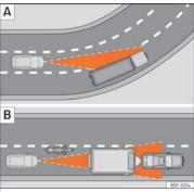
**Fig. 279** A Vehicle on a bend. B Motorcyclist ahead, out of range of the radar sensor.
