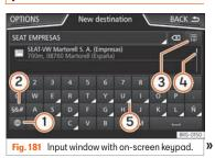
The on-screen keypad is used for functions such as entering an memory name, selecting a destination address or entering a search term for searching long lists.
