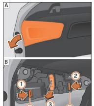
Fig. 65 Remove the cover from the boot lid and detach the bulb holder.
