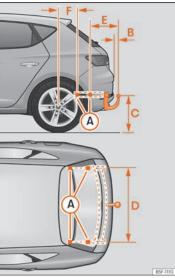
Fig. 307 Limits and attachment points for retrofitting a towing bracket.
