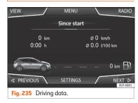
The on-board computer has 3 memories. They can be used to display: distance, time, average speed, average consumption and range.
