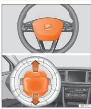
Fig. 15 Driver airbag located in steering wheel.
