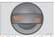
Fig. 318 In the engine compartment: Engine oil filler cap.
