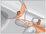
Fig. 102 Driver door handle: lever the cover off
