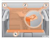
Fig. 160 In the luggage compartment: net partition hooked in place with the rear seat backs folded down.
