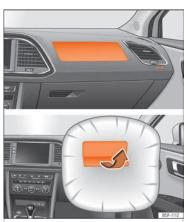
Fig. 16 Front passenger airbag located in dash panel.
