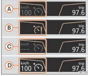
Fig. 267 Instrument panel display: GRA status indications
