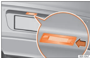
Fig. 121 In the rear bumper: number plate light.
