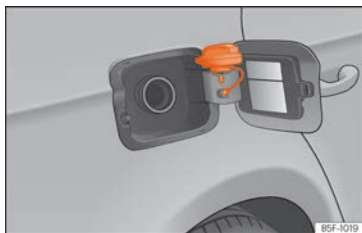
Fig. 61 Fuel tank flap with tank cap attached.
