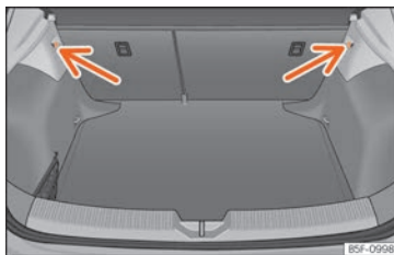
Fig. 187 In the boot: retaining hooks (LEON).
