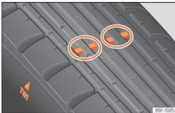
Fig. 313 Tyre profile: tread wear indicators.
