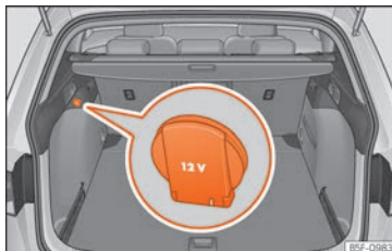
Fig. 170 Detailed view of the side trim in the boot: 12-volt power socket (applies only to the LEON ST model).
