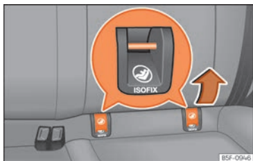
Fig. 39 ISOFIX securing rings.
