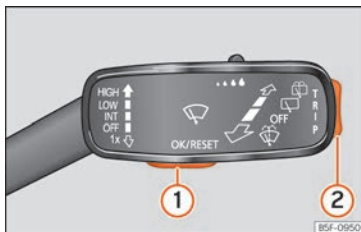
Fig. 136 Windscreen wipers lever: control buttons.
