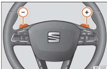
Fig. 260 Steering wheel: automatic gearbox levers
