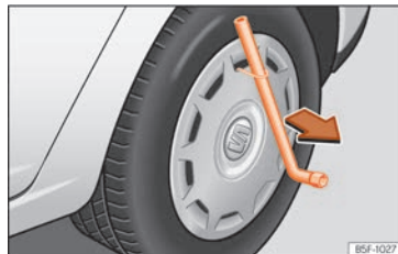
Fig. 74 Remove the wheel cover.
