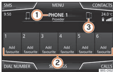
Fig. 244 Telephone main menu (view of the 8" screen).
