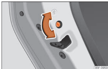
Fig. 147 Childproof lock on the left hand side door.
