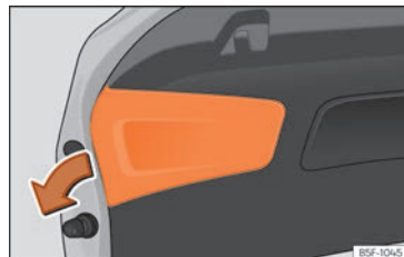
Fig. 119 Remove the cover from the rear lid
