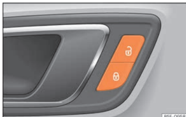
Fig. 5 Driver door: central locking switch.
