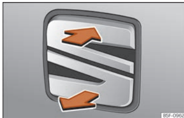
Fig. 8 Rear lid: opening from the outside.
