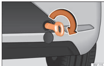
Fig. 103 Right side of the rear bumper: towline anchorage screwed in.
