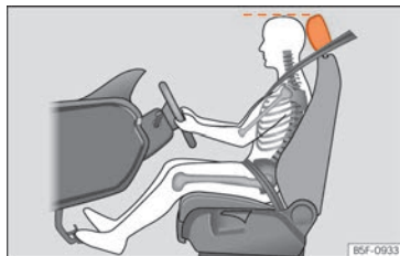
Fig. 88 Correct head restraint position for the driver.
