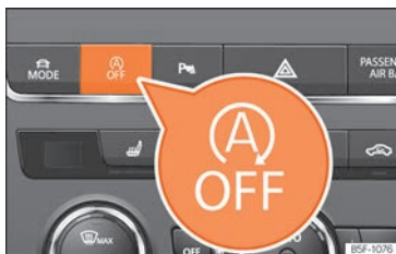
Fig. 262 Centre console: Start-Stop system button.
