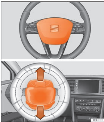
Fig. 26 Driver airbag located in steering wheel.
