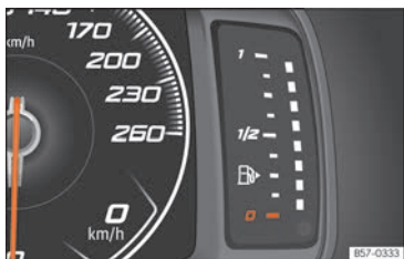
Fig. 132 Digital instrument panel: fuel gauge.
