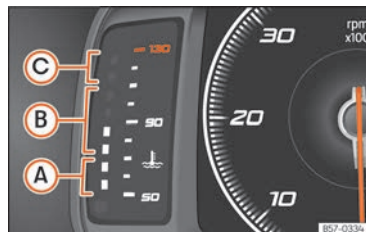
Fig. 135 Digital instrument panel: engine coolant temperature display.
