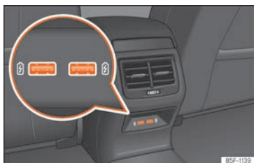
Fig. 248 Centre console, rear section: USB connectors.
