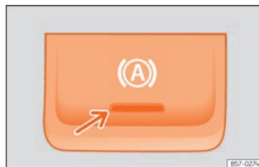
Fig. 263 In the lower part of the centre console: Auto Hold function button.
