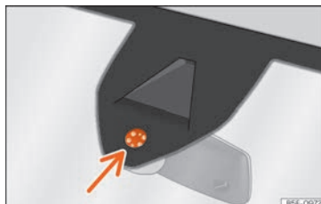
Fig. 157 Rain sensor sensitive surface
