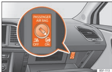
Fig. 28 Front passenger front airbag switch.
