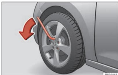
Fig. 185 Wheel: loosen the wheel bolts.
