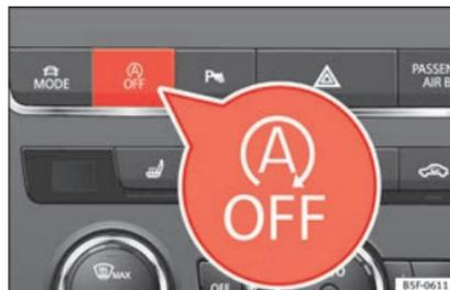
**Fig. 147** Centre console: Start-Stop system button
