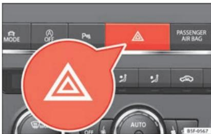
**Fig. 99** Dash panel: switch for hazard warning lights.
