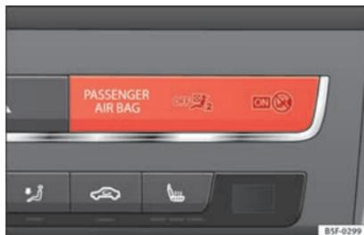
Fig. 73 Control lamp for disabling the front passenger front airbag on the dash panel
