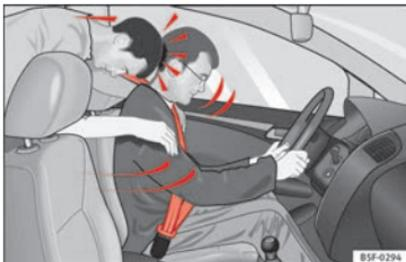
**Fig. 63** The unbelted passenger in the rear seat is thrown forward violently, hitting the driver who is wearing a seat belt.
