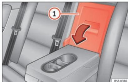
Fig. 128 On the rear seat backrest: opening the tailboard.
