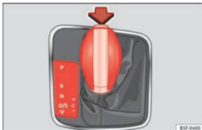
Fig. 143 Selector lever lock.
