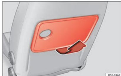
Fig. 114 Left-hand front seat: folding table.
