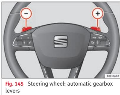
**Fig. 145** Steering wheel: automatic gearbox levers
