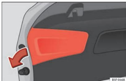
Fig. 220 Remove the cover from the boot lid.
