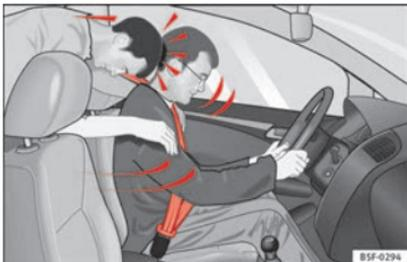
**Fig. 61** Drivers with properly worn seat belts will not be thrown forward in the event of sudden braking
