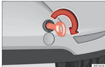
**Fig. 193** Right side of the rear bumper: towline anchorage screwed in.
