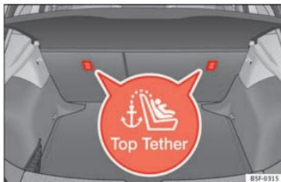
**Fig. 79** Position of the Top Tether rings on the back of the rear seat.
