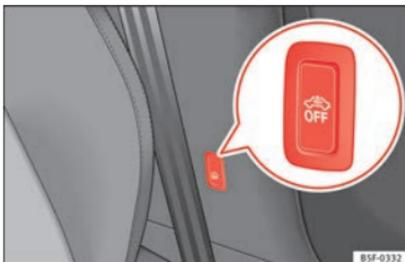
Fig. 96 Vehicle interior monitoring/tow-away protection button.
