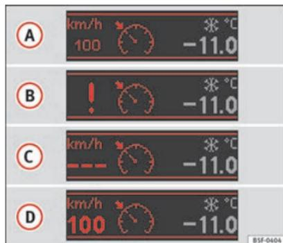
Fig. 148 Instrument panel display: CCS status indications
