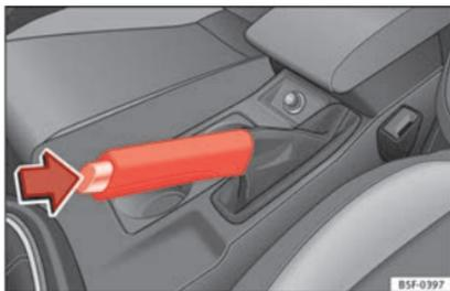
Fig. 142 Handbrake between the front seats.
