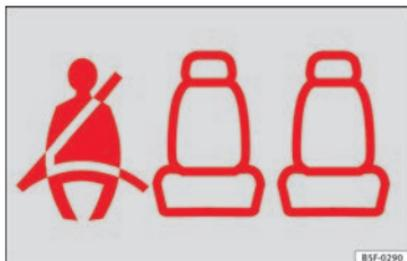
**Fig. 60** Instrument panel: right rear seat occupied and corresponding seat belt fastened display.
