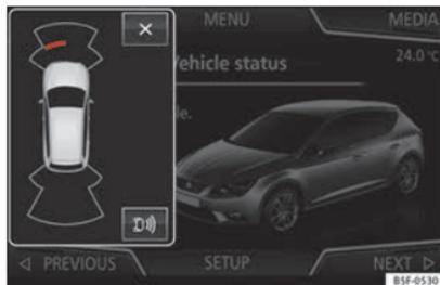
Fig. 170 Miniature indication of automatic activation
