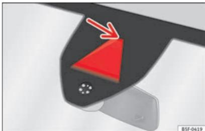
**Fig. 164** In the windscreen: field of vision of the Lane Assist system camera.
