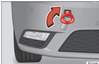
**Fig. 191** Right side of the front bumper: towline anchorage screwed in.
