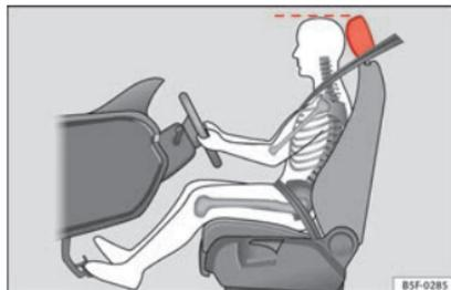
**Fig. 56** Correct head restraint position for the driver.
