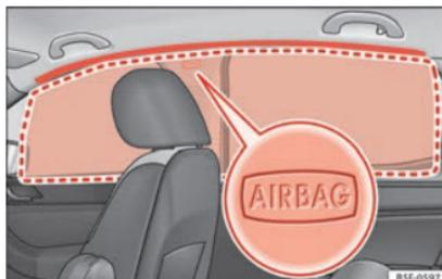
Fig. 72 Location of head-protection airbags.
