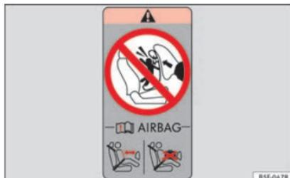
**Fig. 77** On the rear frame of the passenger side door: airbag sticker.
