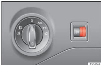
**Fig. 100** Next to the steering wheel: Headlight range control
