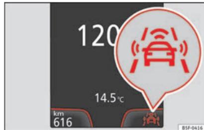
Fig. 160 On the instrument panel display: Front Assist switched off message.
