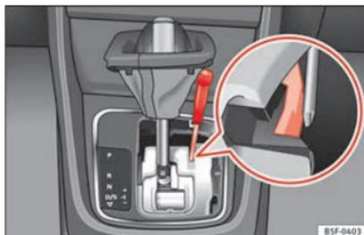
**Fig. 198** Selector lever: manual release from position P.
