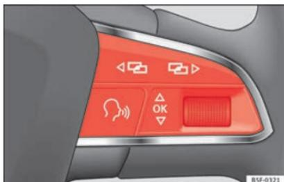
**Fig. 88** Right side of multifunction steering wheel: control buttons.
