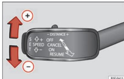
**Fig. 153** On the left of the steering column: third lever for operating the Adaptive Cruise Control.
