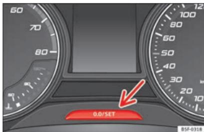
Fig. 84 Instrument panel: odometer and reset button.
