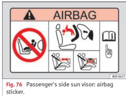
**Fig. 76** Passenger's side sun visor: airbag sticker.
