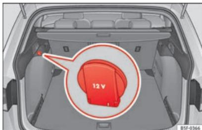
Fig. 118 Detailed view of the side trim in the luggage compartment: 12-volt power socket (applies only to the LEON ST model).
