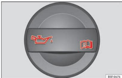
**Fig. 176** In the engine compartment: Engine oil filler cap
