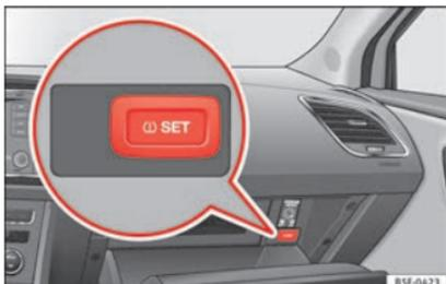
**Fig. 180** Glove compartment: tyre control switch.
