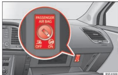
Fig. 74 Front passenger front airbag switch.
