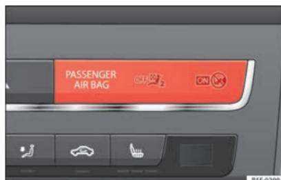
Fig. 75 Warning lamp for disabling the front passenger airbag.
