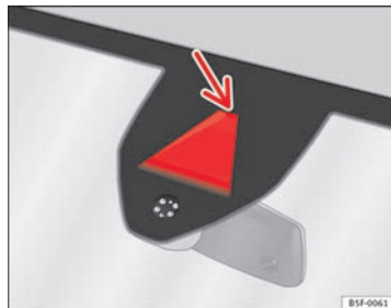
Fig. 99 In the windscreen: Field of vision of the Lane Assist system camera
