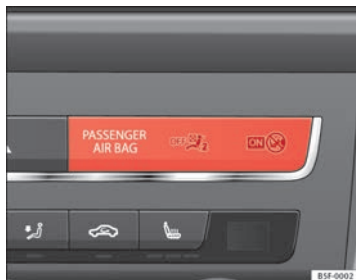
Fig. 16 Control lamp for disabling the front passenger front airbag on the dash panel
