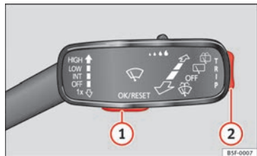
Fig. 40 Vehicles without multifunction steering wheel: Button ① on the windscreen wiper lever to confirm the menu options and rocker switch ② to change menu
