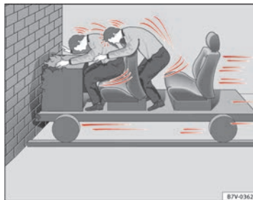
Fig. 7 The vehicle hits the wall: the occupants are not wearing seat belts
