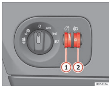
Fig. 73 Dash panel: regulation for instrument and switch illumination and headlight range control
