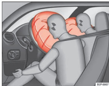
Fig. 19 Inflated front airbags
