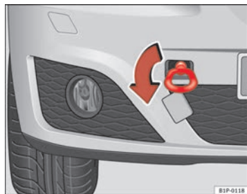
Fig. 183 The front right section of the vehicle: Fitting the front towing eye
