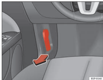
Fig. 142 Detail of foot-well area on driver side: lever for unlocking the bonnet.
