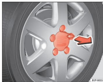
Fig. 155 Changing the wheel: Removing a hub cap
