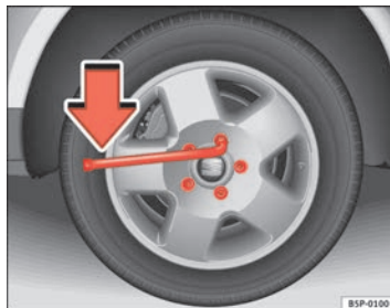
Fig. 156 Changing the wheel: loosen the wheel bolts
