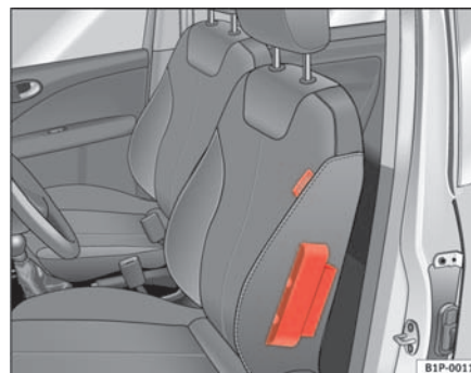
Fig. 21 Side airbag in driver seat
