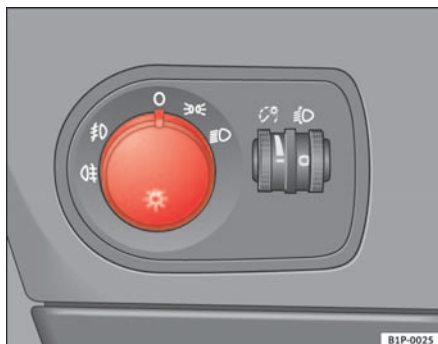
Fig. 72 Detail of the dash panel: Switch for lights, fog lights and rear fog light
