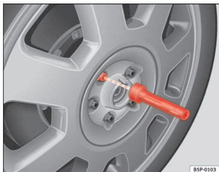
Fig. 158 Wheel change: Hexagon socket in screwdriver handle to turn the wheel bolts after they have been loosened
