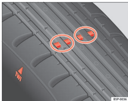
Fig. 151 Tyre tread wear indicators
