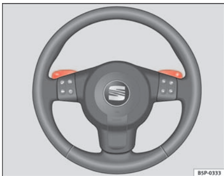
Fig. 123 Steering wheel with levers for the automatic gearbox
