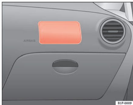
Fig. 18 Front passenger airbag located in dash panel
