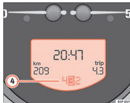
Fig. 36 Detail of instrument panel: Display with Tiptronic gear selection
