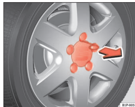
Fig. 154 Changing a wheel: Removing the wheel trim
