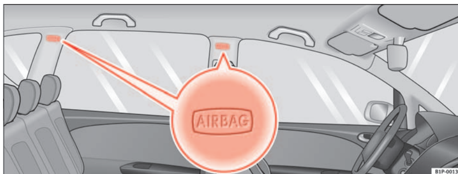
Fig. 23 Location of left curtain airbag
