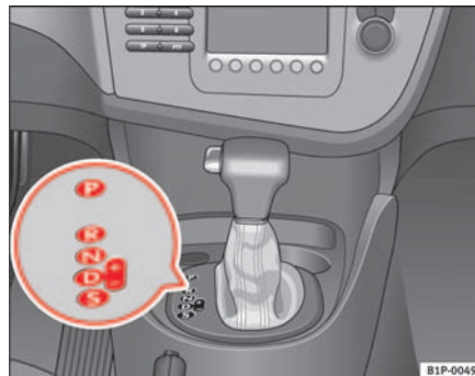
Fig. 115 Section of centre console: selector lever on cars with an automatic gearbox / direct shift gearbox
