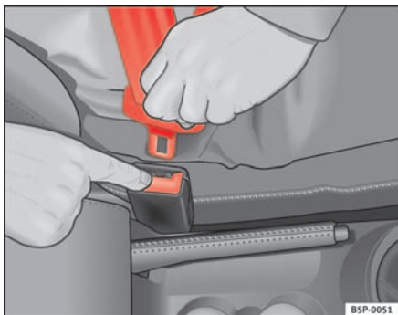
Fig. 15 Removing latch plate from buckle
