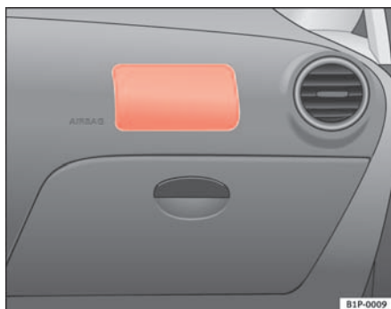
Fig. 18 Front passenger airbag located in dash panel
