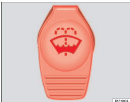
Fig. 139 In the engine compartment: Cap of windscreen washer fluid reservoir.
