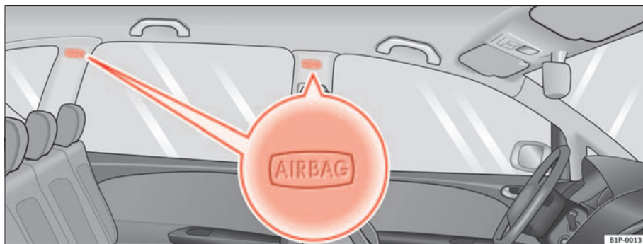
Fig. 23 Location of left curtain airbag
