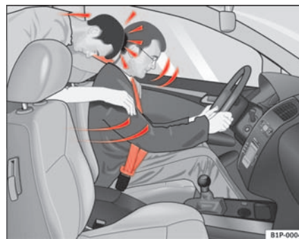
Fig. 9 The unbelted rear passenger is thrown forward violently, hitting the driver wearing a seat belt.
