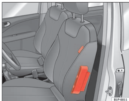
Fig. 21 Side airbag in driver seat
