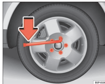
Fig. 147 Changing the wheel: Loosening the wheel bolts
