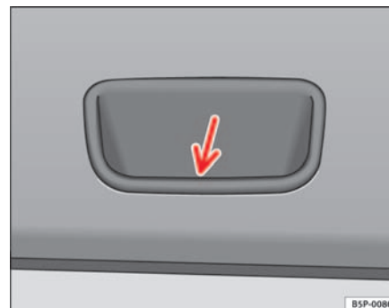
Fig. 66 Detail of the tailgate inner trim: recessed handle for closing the tailgate
