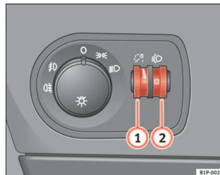
Fig. 74 Detail of the dash panel: Regulation for instrument and switch illumination and headlight range control
