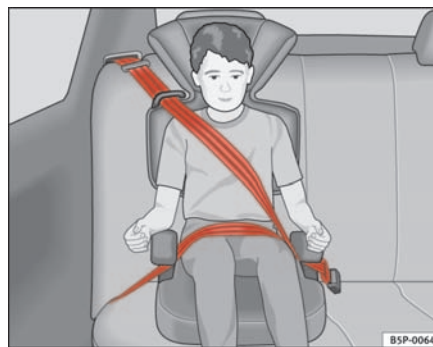
Fig. 29 Forward-facing child seat installed on rear seat.
