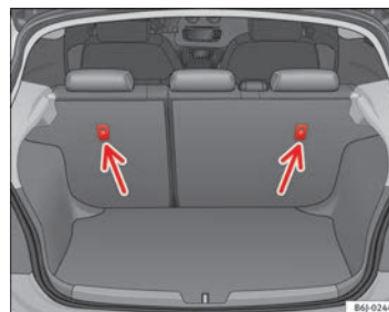
Fig. 27 Position of the Top Tether rings on the back of the rear seat
