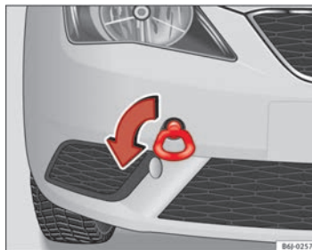
Fig. 171 Fitting the towline anchorage to front of the vehicle
