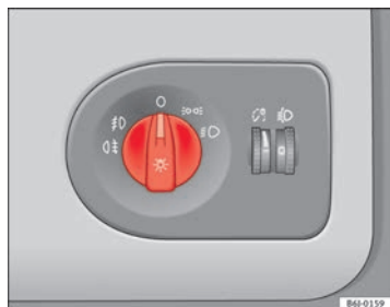
Fig. 53 Detailed view of the dash panel: lights, fog lights and rear fog light switch
