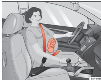
Fig. 14 Positioning seat belts during pregnancy ▶
