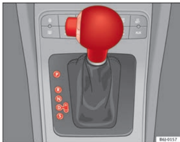
Fig. 107 Changing gear with tiptronic
