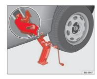
Fig. 129 Fitting the jack
