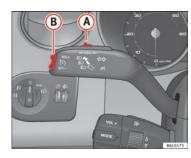
Fig. 109 Turn signal and main beam headlight lever: switch and rocker switch for the cruise
