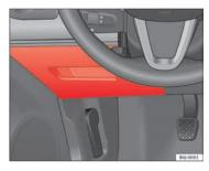
Fig. 132 Fuses in the dash panel
