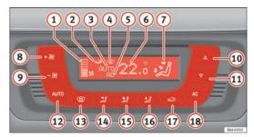
Fig. 92 Climatronic controls on the dash panel
