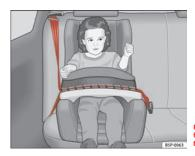
Fig. 24 A category 1 forward-facing child seat fitted on the rear seat.
