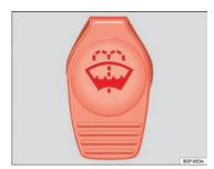
Fig. 120 In the engine compartment: Cap of windscreen washer fluid reservoir.
