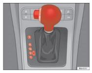
Fig. 103 Changing gear with tiptronic
