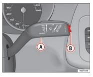
Fig. 34 Windscreen wiper and windscreen wash lever: button A and rocker switch B
