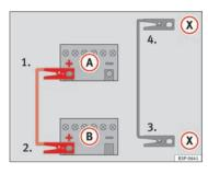
Fig. 155 Diagram for connecting jump leads if the vehicle providing assistance is fitted with the Start-Stop system: flat battery (a) and battery providing current (a).
