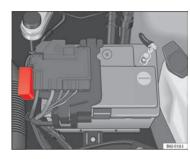
Fig. 133 Fuses in engine compartment
