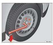
Fig. 127 Changing the wheel: loosen the wheel bolts
