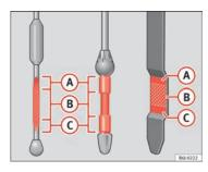
Fig. 117 Engine oil dipstick
