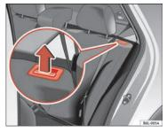
Fig. 72 Button for unlocking the rear backrest
