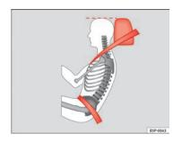
Fig. 67 Side view: head restraints and seat belts correctly adjusted
