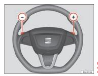
Fig. 104 Steering wheel with paddle levers for automatic gearbox
