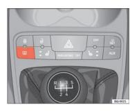
Fig. 55 Centre console: heated rear window switch
