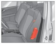
Fig. 19 Side airbag in driver seat
