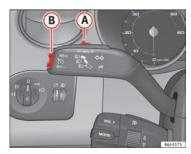
Fig. 111 Turn signal and main beam headlight lever: switch and rocker switch for the cruise control
