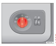
Fig. 51 Detailed view of the dash panel: lights, fog lights and rear fog light switch
