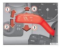
Fig. 57 Turn signal and main beam headlight lever
