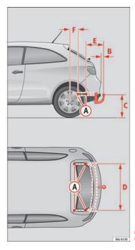
Fig. 113 Attachment points for towing bracket
