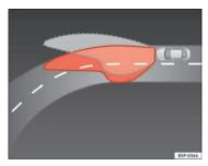
Fig. 54 Cornering lighting using adaptive headlights
