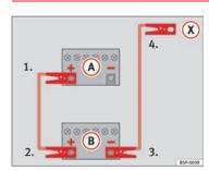
Fig. 154 Diagram for connecting jump leads if the vehicle providing assistance the current is not fitted with the Start-Stop system: flat battery (A) and battery providing current (B).
