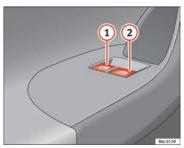
Fig. 48 Detail of the driver door: controls for the front windows.
