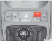
Fig. 94 Detailed view of the centre console: ESP button
