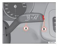
Fig. 33 Windscreen wiper lever: button A and rocker switch B
