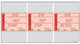
Fig. 97 Display on the instrument panel during Start-Stop function operation.
