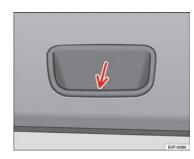
Fig. 46 Detail of the inside of the tailgate: hand grip
