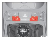
Fig. 70 Front seats heating switch
