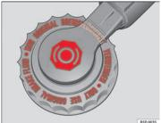
Fig. 123 In the engine compartment: Brake fluid reservoir cover
