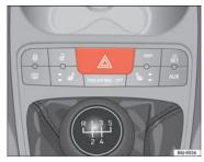
Fig. 56 Centre console: switch for hazard warning
