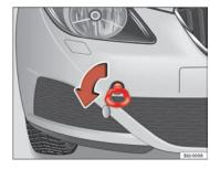
Fig. 156 Fitting the towing eye to front rear of the vehicle
