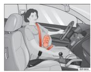
Fig. 14 Positioning seat belts during pregnancy
