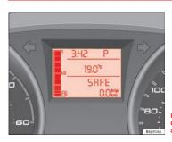
Fig. 35 Digital display: Gear lever position for automatic gearbox.
