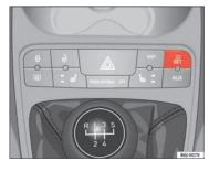
Fig. 38 Centre console: tyre monitor system button
