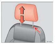
Fig. 68 Adjusting and removing the head restraints
