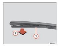
Fig. 122 Changing the rear window wiper blade
