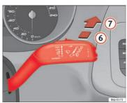
Fig. 63 Windscreen wiper and windscreen wash lever: rear window wiper
