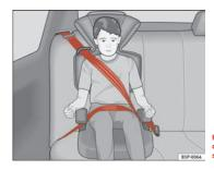
Fig. 25 Forward-facing child seat installed on rear seat.
