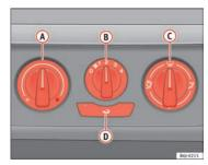
Fig. 87 Heating controls on the dash panel
