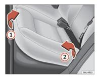
Fig. 71 Folding up the rear seat cushion
