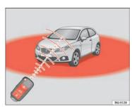
Fig. 44 Range of the remote control
