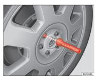
Fig. 130 Changing the wheel: Hexagonal socket in screwdriver handle to turn the wheel bolts
