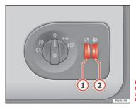
Fig. 53 Dash panel: regulation for instrument and switch illumination and headlight range control
