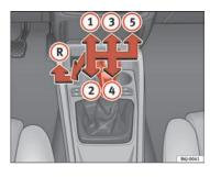
Fig. 98 Centre Console: gear shift pattern of a 5speed manual gearbox
