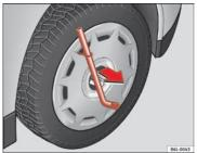
Fig. 126 Remove the complete hub cap
