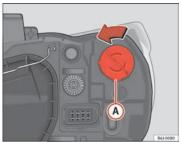
Fig. 141 Single turn signal lamp
