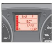
Fig. 101 Automatic gearbox: Instrument panel display
