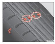
Fig. 124 Tyre tread wear indicators
