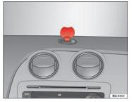
Fig. 76 Bracket with open cover for placing the navigator.
