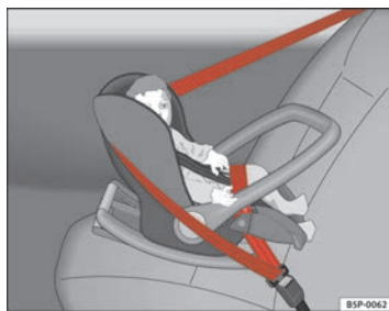
Fig. 25 A group 0 rear-facing child seat fitted on the rear seat.
