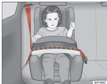
Fig. 26 A category 1 forward-facing child seat fitted on the rear seat.
