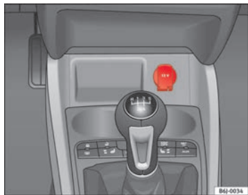
Fig. 82 Front power point
