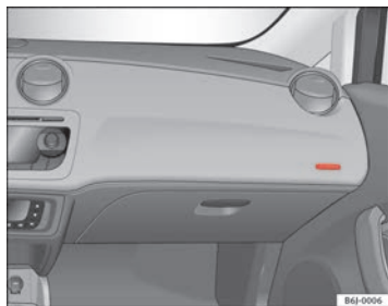
Fig. 17 Front passenger airbag located in dash panel
