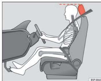
Fig. 2 Proper head restraint position for driver
