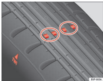
Fig. 121 Tyre tread wear indicators
