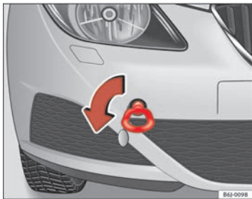
Fig. 152 Fitting the towing eye to the front of the vehicle
