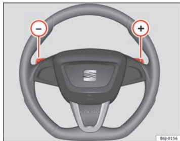
Fig. 101 Steering wheel with paddle levers for automatic gearbox
