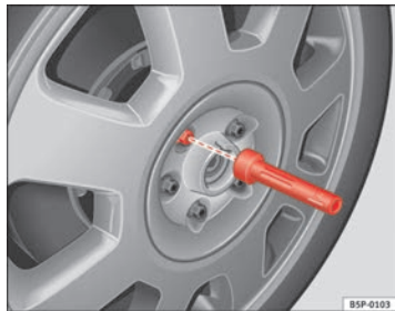
Fig. 127 Changing the wheel: Hexagonal socket in screwdriver handle to turn the wheel bolts
