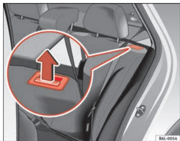
Fig. 71 Button for unlocking the rear backrest
