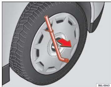
Fig. 123 Remove the complete hub cap
