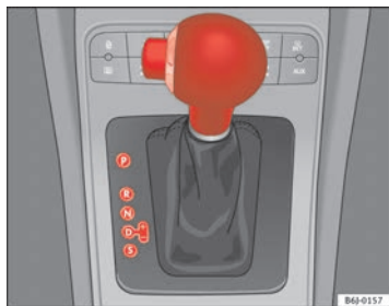
Fig. 100 Changing gear with Tiptronic
