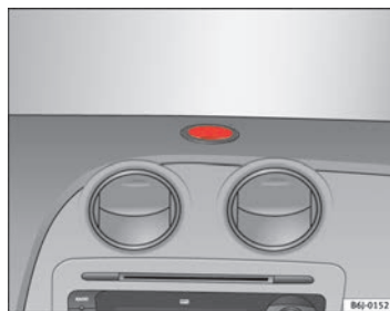
Fig. 74 Mounting bracket for navigator in instrument panel.
