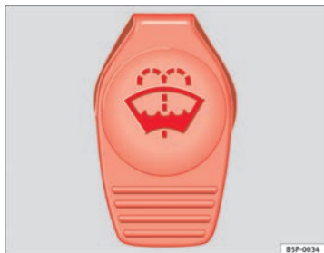
Fig. 117 In the engine compartment: Cap of windscreen washer fluid reservoir.
