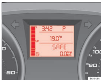
Fig. 35 Digital display: Selector lever position for the automatic gearbox.
