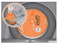
Fig. 183 In the boot: remove the subwoofer.
