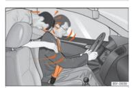
Fig. 23 Any rear seat occupants not wearing a seat belt may be thrown forward violently, hitting the driver who is wearing the seat belt.
