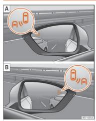
**Fig. 115** Control lamp of the lane departure warning.
