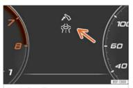
**Fig. 12** Eco-efficient driving assistance indication (schematic representation).
