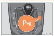
**Fig. 120** Centre console: parking aid button (depending on the version).
