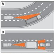
**Fig. 107** A Vehicle on a bend. B Motorcyclist ahead, out of range of the radar sensor.
