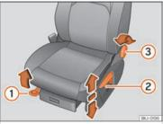
Fig. 66 Front seats: manual seat adjustment.
