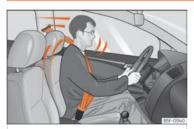
Fig. 20 Drivers with properly worn seat belts will not be thrown forward in the event of sudden braking.
