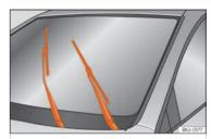
Fig. 150 Wipers in service position.
