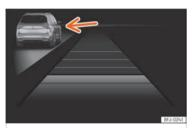
**Fig. 106** On the instrument panel display: ACC active, vehicle detected on the left.
