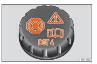
Fig. 173 Engine compartment: brake fluid reservoir cap.
