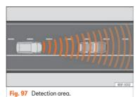
A radar sensor may be fitted to the front bumper of the vehicle » Fig. 96. The front radar detects any objects in its detection zone » Fig. 97 and provides support for the following functions:
