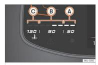
Fig. 8 Basic digital instrument cluster; engine coolant temperature displau.
