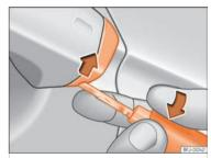
**Fig. 55** Driver's door handle: pry the cover open.
