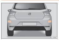
Fig. 99 Rear view of the vehicle: radar sensor areas.
