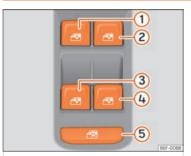
**Fig. 60** Detail of the driver door: controls for the windows.
