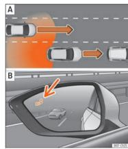
Fig. 116 Schematic diagram: A Overtaking with traffic behind the vehicle. Side Assist indication on the left hand side
