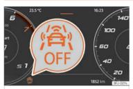
**Fig. 111** On the screen of the instrument panel Front Assist switched off message.
