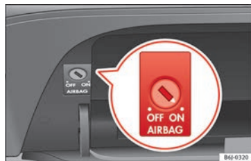
Fig. 85 In the glove compartment: Switch for activating and deactivating the front passenger airbag
