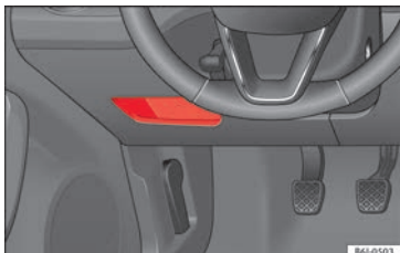
Fig. 57 On the driver-side dash panel: fuse box cover
