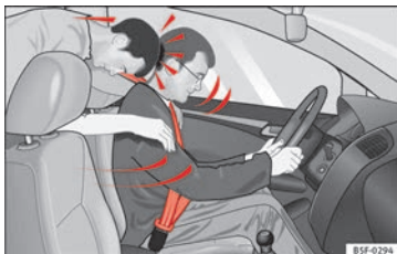
Fig. 82 The unbelted passenger in the rear seat is thrown forward violently, hitting the driver who is wearing a seat belt.
