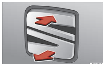
Fig. 3 Rear lid: opening from the outside.
