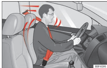
Fig. 80 Drivers with properly worn seat belts will not be thrown forward in the event of sudden braking
