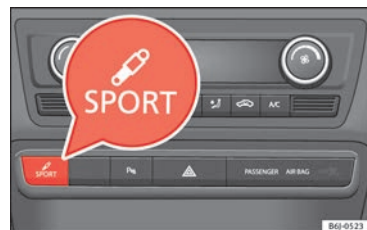
Fig. 183 In the centre console: button to adjust the “SEAT Drive Profile” system
