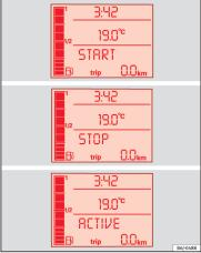
Fig. 142 Display on the instrument panel during Start-Stop function operation.
