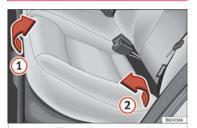
Fig. 101 Folding up the rear seat cushion.
