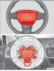
Fig. 56 Driver airbag located in steering wheel.
