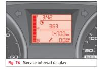
The service indication is shown on the instrument panel display **»» Fig. 76**.
