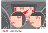
Use the gear display to save fuel. If you are not in the correct gear, a triangle will appear next to the gear display indicating whether you should change up or down >>> Fig. 73. For further information on the gear change display, please see the >>> page 134.
