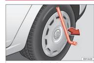
Fig. 158 Remove the wheel cover.
