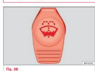
The windscreen washer reservoir is located in the engine compartment >>> page 168.
