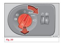
Turn the switch to the required position **>>> Fig. 20**.
