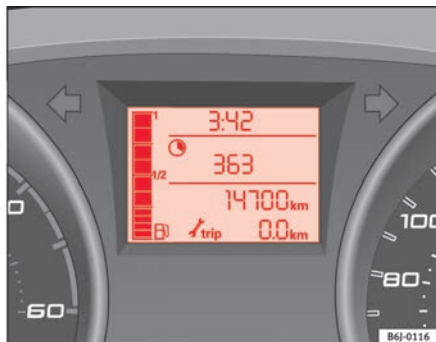
Fig. 35 Service interval display
