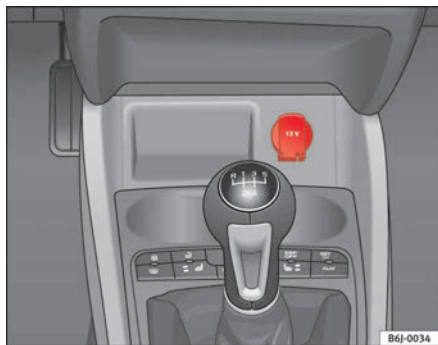
Fig. 82 Front power point
