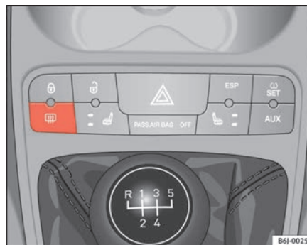
Fig. 54 Centre console: heated rear window switch
