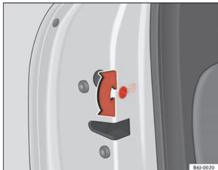
Fig. 41 Child safety lock on the left hand side door
