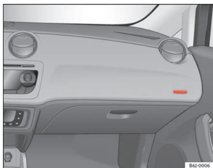
Fig. 17 Front passenger airbag located in dash panel
