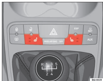
Fig. 69 Front seats heating switch
