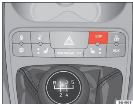
Fig. 93 Detail of the centre console: ESP button
