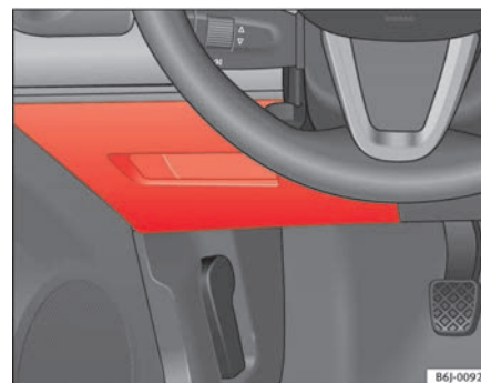
Fig. 141 Fuses in the dash panel
