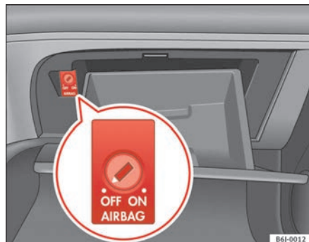
Fig. 23 In the glovebox: key for enabling and disabling front passenger airbag
