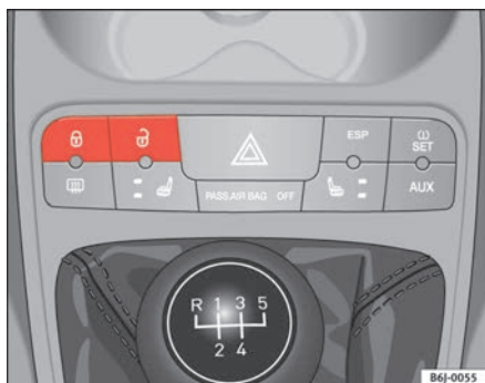
Fig. 40 Central locking button
