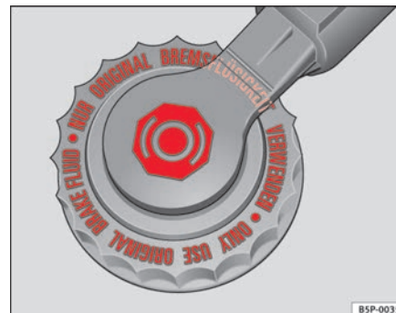
Fig. 132 In the engine compartment: Brake fluid reservoir cover
