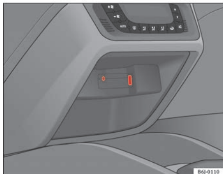
Fig. 84 AUX /USB* input connection (depending on the equipment)
