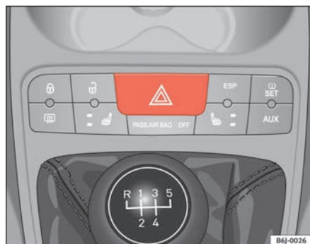
Fig. 55 Centre console: switch for hazard warning lights
