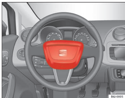
Fig. 16 Driver airbag located in steering wheel
