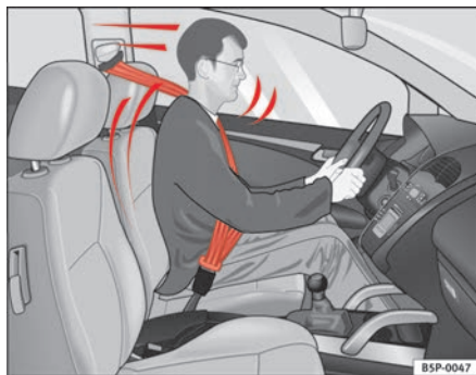
Fig. 10 Driver wearing the seat belt properly: is secured by the belt in sharp braking
