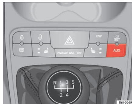
Fig. 83 AUX connection on the central console (depending on the equipment)
