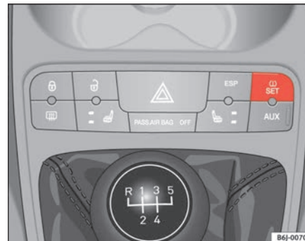
Fig. 37 Centre console: tyre monitor system button
