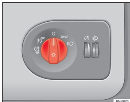
Fig. 51 Detailed view of instrument panel: lights, fog light and rear fog light control
