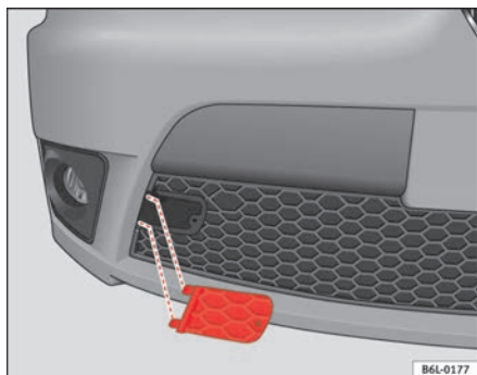
Fig. 173 Eye cover in the lower front grille.
