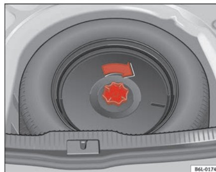
Fig. 138 Securing the defective wheel in the spare wheel well
