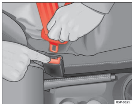
Fig. 15 Removing latch plate from buckle
