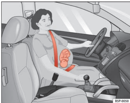
Fig. 14 Positioning seat belts during pregnancy
