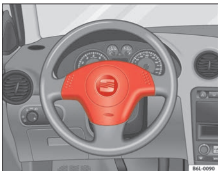
Fig. 17 Driver airbag located in steering wheel
