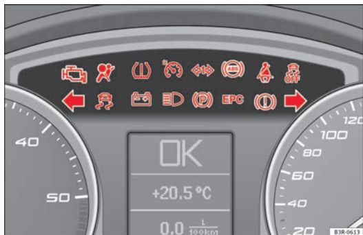
Fig. 45 Instrument panel with warning and indicator lamps
