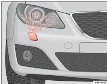
Fig. 102 Headlight with extended washer jet
