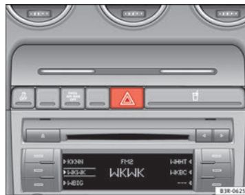
Fig. 91 Centre console: Switch for hazard warning lights
