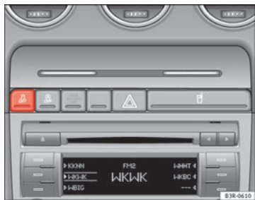
Fig. 164 Centre console with ESC switch
