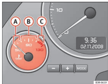
Fig. 39 Engine coolant temperature gauge
