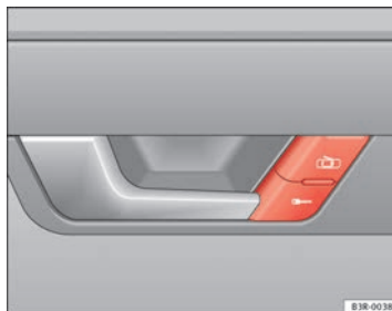
Fig. 72 Detail of the driver door: Central locking switch
