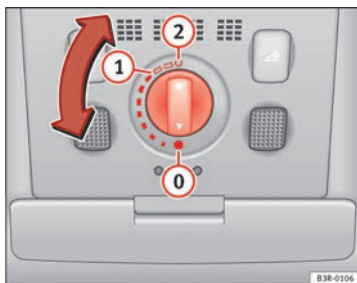
Fig. 83 Detail of headliner: Sliding/tilting sunroof control
