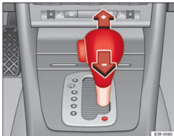
Fig. 161 Centre console: Manual gear selection (tiptronic mode)
