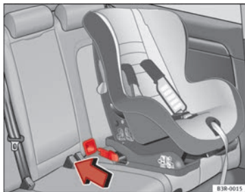
Fig. 34 The ISOFIX child seat anchors slide along the fitted plastic guides until secured in the vehicle's ISOFIX anchorages
