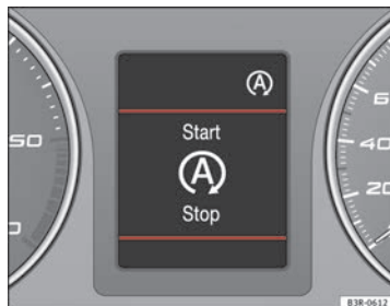
Fig. 149 Display on the instrument panel during Start-Stop function operation.
