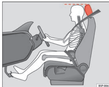
Fig. 2 Correct head restraint position for driver
