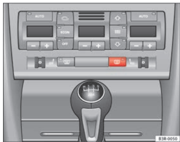
Fig. 97 Switch for heated rear window
