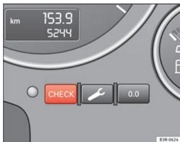
Fig. 54 Instrument panel: CHECK button
