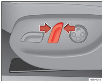
Fig. 108 Front seat: Backrest adjuster switch
