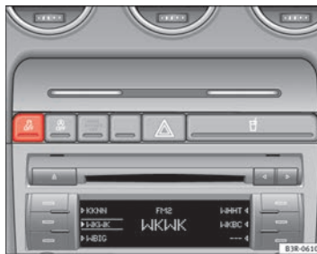
Fig. 145 Detailed view of the centre console: ESC button
