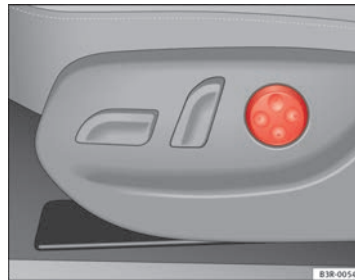
Fig. 109 Front seat: Ad- juster switch for lumbar support
