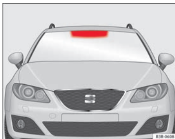
Fig. 177 Location of the electronic toll collection system
