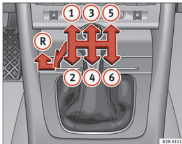
Fig. 157 Detailed view of the centre console: gear shift pattern of a 6-speed manual gearbox
