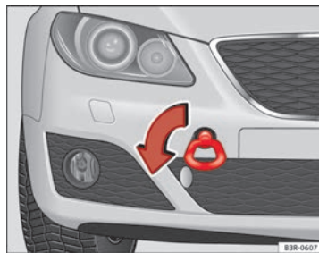
Fig. 247 Fitting the towline anchorage to front of the vehicle
