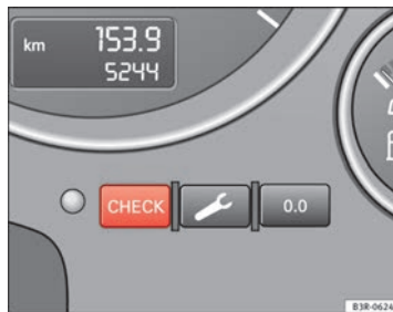
Fig. 58 Detailed view of the instrument panel: CHECK button
