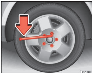
Fig. 197 Changing a wheel: Loosen the wheel bolts
