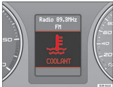
Fig. 55 Display: Coolant level warning
