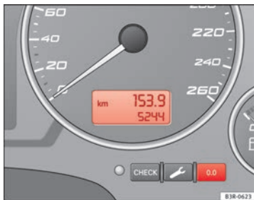
Fig. 43 Detailed view of the instrument panel: Odometer
