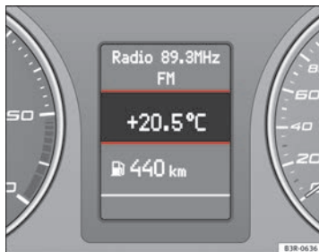
Fig. 50 Display: Outside temperature indicator
