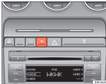
Fig. 154 Centre console: switch for parking aid
