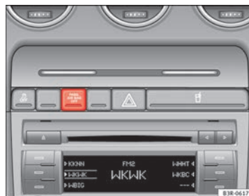
Fig. 29 Control lamp for deactivated front passenger airbag in centre console
