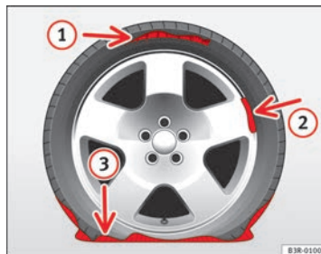
Fig. 201 The Tyre Mobility System is not suitable for repairing this type of damage to tyres.
