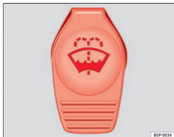
Fig. 184 In the engine compartment: Cap of windscreen washer fluid reservoir
