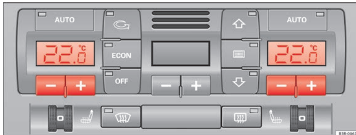
Fig. 140 Air conditioner controls
