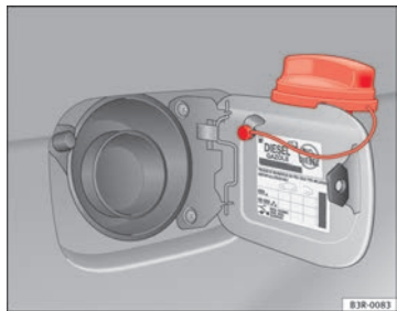
Fig. 178 Fuel tank flap with tank cap attached
