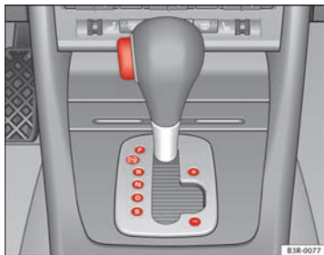
Fig. 158 Detailed view of the centre console: Selector lever with lock button
