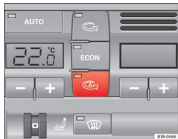
Fig. 141 Button for automatic air recirculation
