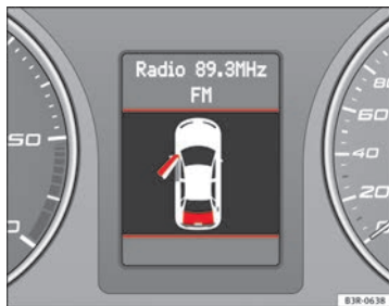
Fig. 52 Display: Door and rear lid warning
