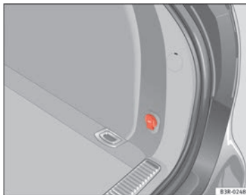
Fig. 135 Detailed view of the side trim in the luggage compartment: 12 volt power socket
