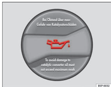
Fig. 182 In the engine compartment: Engine oil filler cap
