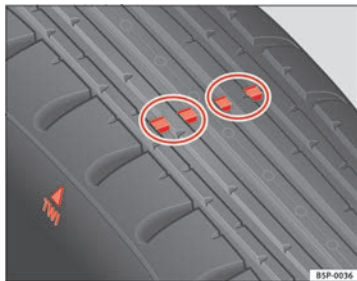
Fig. 191 Tyre tread wear indicators
