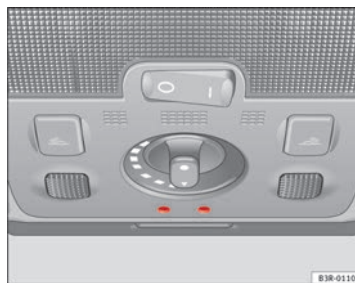
Fig. 94 Detail of headliner: Ambient lighting
