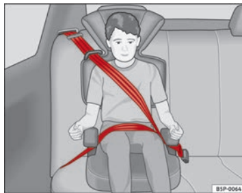
Fig. 32 Forward-facing child seat installed on rear seat
