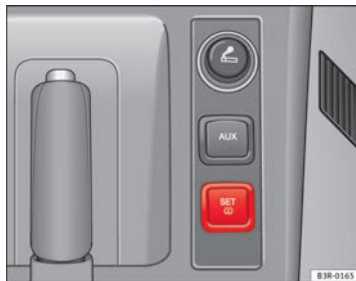
Fig. 190 Detailed view of the centre console: Button for the tyre pressure monitoring system
