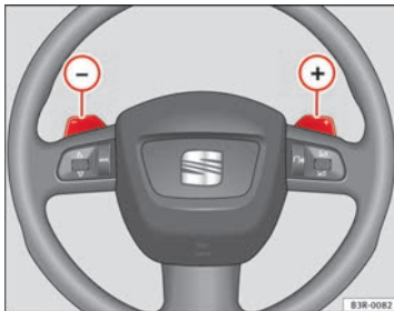
Fig. 163 Steering wheel: tiptronic controls
