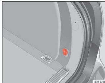
Fig. 134 Detailed view of the side trim in the luggage compartment: 12 volt socket
