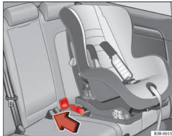
Fig. 33 The ISOFIX child seat anchors slide along the fitted plastic guides until secured in the vehicle's ISOFIX anchorages
