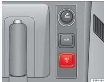
Fig. 189 Detailed view of the centre console: Button for the tyre pressure monitoring system
