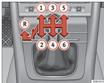
Fig. 156 Detailed view of the centre console: gear shift pattern of a 6-speed manual gearbox
