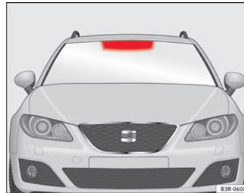
Fig. 176 Location of the electronic toll collection system
