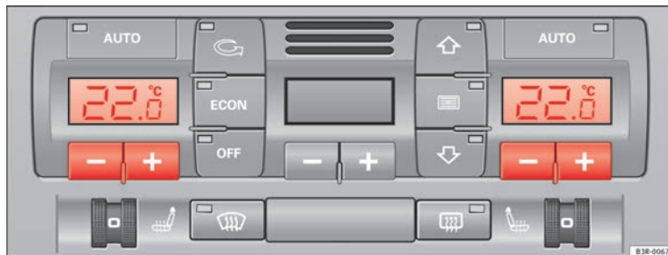
Fig. 139 Air conditioner controls
