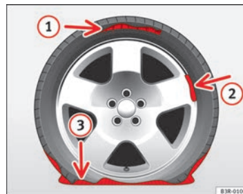
Fig. 200 The Tyre Mobility System is not suitable for repairing this type of damage to tyres.
