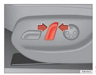
Fig. 109 Front seat: Backrest adjuster switch
