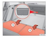
Fig. 75 Detail of the rear seats and luggage compartment: access to the emergency release mechanism
