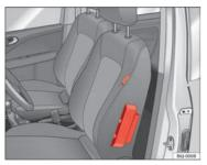
Fig. 23 Side airbag in driver seat
