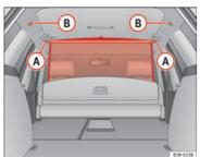
Fig. 121 Retainers for the net partition
