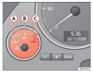
Fig. 38 Engine coolant temperature gauge
