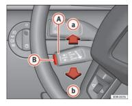
Fig. 152 Controls for the cruise control system
