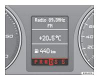
Fig. 155 Display: Selector lever positions
