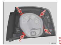
Fig. 225 Securing the bulb holder in the tail light unit
