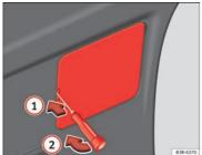
Fig. 230 Remove the cover of the tailgate trim
