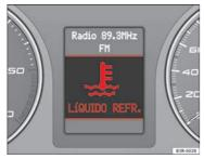
Fig. 54 Display: Coolant level warning
