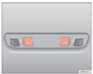
Fig. 96 Detail of headliner: rear reading lights
