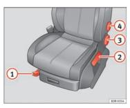
Fig. 106 Adjuster controls on driver seat
