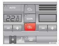
Fig. 142 Button for automatic air recirculation
