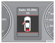
Fig. 51 Display: Door and tailgate warning
