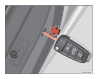
Fig. 73 Activating manual locking
