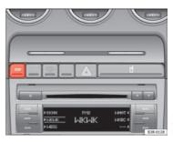
Fig. 146 Detailed view of the centre console: ESP button
