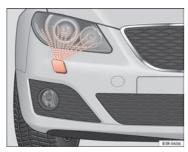
Fig. 103 Headlight with extended washer jet
