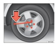
Fig. 193 Changing the wheel: Loosen the wheel bolts
