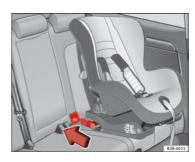
Fig. 33 The ISOFIX child seat anchors slide along the fitted plastic guides until secured in the vehicle's ISOFIX anchorages
