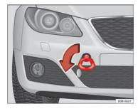
Fig. 242 Fitting the towing eye to front rear of the vehicle
