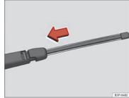
Fig. 184 Fitting the rear window wiper blade
