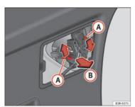
Fig. 231 Remove the bulb holder
