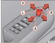
Fig. 105 Detailed view of the armrest: Adjuster
