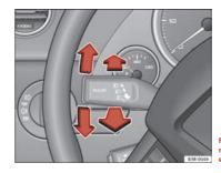
Fig. 93 Turn signal and main beam headlight lev-
