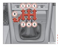
Fig. 153 Detailed view of the centre console: gear shift pattern of a 6-speed manual gearbox
