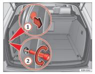
Fig. 220 Luggage compartment: Location of the bolt securing the tail light unit
