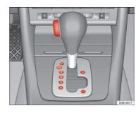
Fig. 154 Detailed view of the centre console: Selector lever with lock but-
