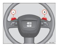
Fig. 159 Steering wheel: tiptronic controls
