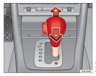
Fig. 157 Centre console: Manual gear selection (tiptronic mode)
