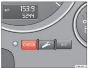
Fig. 53 Instrument panel: CHECK button
