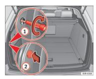
Fig. 227 Luggage compartment: Location of the bolt securing the tail light unit
