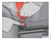
Fig. 15 Removing latch plate from buckle
