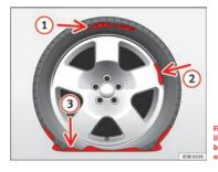
Fig. 197 The Tyre Mobility System is not suitable for repairing this type of damage to tyres.
