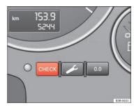
Fig. 57 Detailed view of the instrument panel: CHECK button
