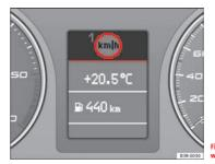
Fig. 56 Display: Speed warning function
