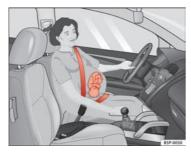
Fig. 14 Positioning seat belts during pregnancy
