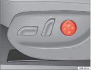
Fig. 110 Front seat: Adjuster switch for lumbar support
