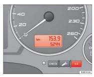
Fig. 42 Detailed view of the instrument panel: Odometer
