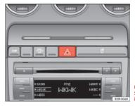
Fig. 92 Centre console: Switch for hazard warning lights
