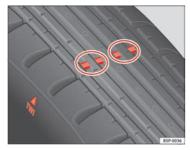
Fig. 187 Tyre tread wear indicators
