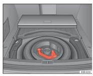
Fig. 162 Luggage compartment: Spare wheel with towing bracket
