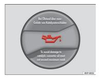
Fig. 178 In the engine compartment: Engine oil filler cap
