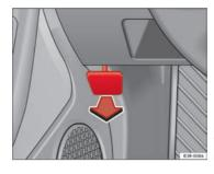
Fig. 175 Detail of footwell area on driver side: lever for unlocking the bonnet.
