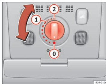
Fig. 82 Details of headliner: Rotary sun roof control
