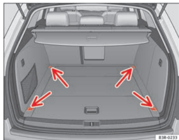
Fig. 117 Location of fastening rings in luggage compartment
