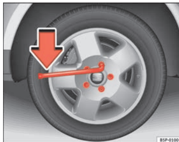
Fig. 195 Changing the wheel: Loosen the wheel bolts
