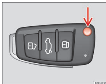
Fig. 67 Remote control key: Release button
