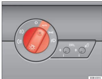
Fig. 86 Detailed view of instrument panel: Light switch
