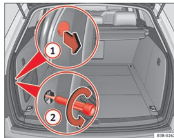
Fig. 225 Luggage compartment: Location of the bolt securing the rear light
