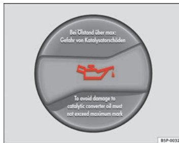
Fig. 180 In the engine compartment: Engine oil filler cap
