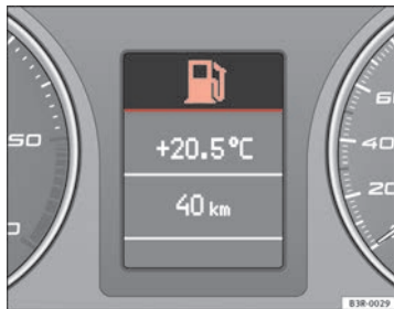
Fig. 55 Display: Fuel level low
