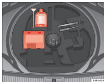
Fig. 193 Tyre Mobility System under floor panel in luggage compartment
