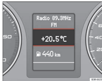
Fig. 49 Display: Ambient temperature display
