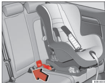
Fig. 33 The ISOFIX child seat anchorings slide along the fitted plastic guides until secured in the vehicle's ISOFIX anchorages
