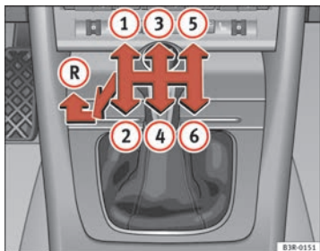
Fig. 153 Detail of the centre console: gear shift pattern of a 6-speed manual gearbox
