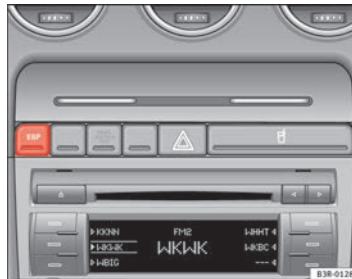
Fig. 146 Detail of the centre console: ESP button
