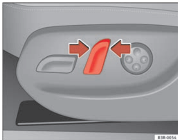
Fig. 109 Front seat: Backrest adjuster switch
