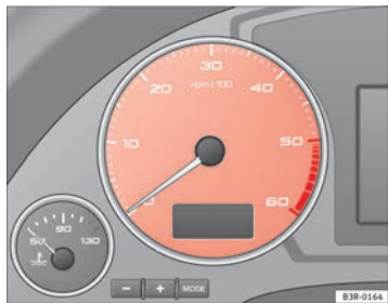
Fig. 39 Detailed view of the dash panel insert: Rev. counter
