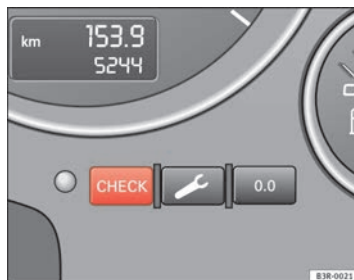
Fig. 57 Detail of the dash panel insert: CHECK button
