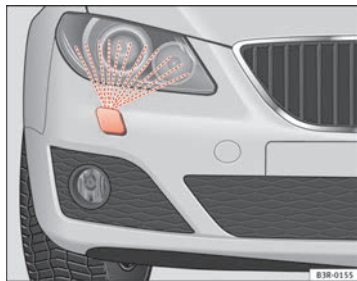
Fig. 103 Headlight with extended washer jet
