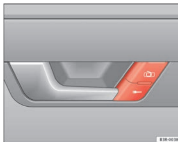
Fig. 71 Detail of driver door: Central locking switch
