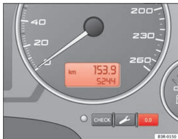
Fig. 42 Detail of the dash panel insert: Distance display
