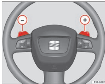
Fig. 159 Steering wheel: Tiptronic controls
