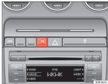
Fig. 150 Centre console: switch for parking aid
