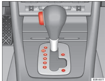
Fig. 154 Detail of the centre console: Selector lever with lock button
