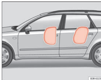
Fig. 24 Inflated side airbag on left side of vehicle
