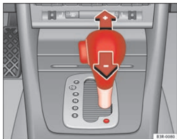
Fig. 157 Centre console: Manual gear selection (tiptronic mode)
