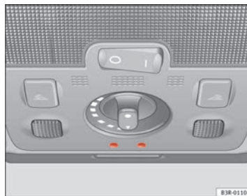
Fig. 95 Details of headliner: background lighting
