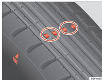
Fig. 189 Tyre tread wear indicators
