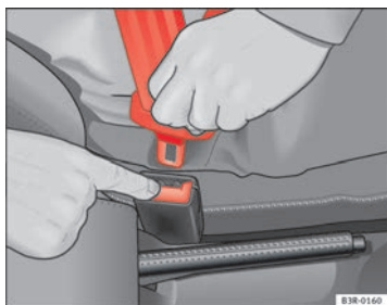
Fig. 15 Removing latch plate from buckle
