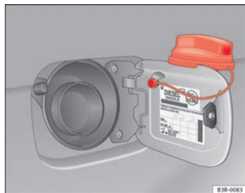
Fig. 174 Fuel tank flap with tank cap attached
