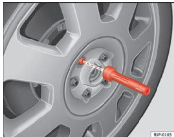
Fig. 198 Changing the wheel: Hexagonal socket in screwdriver handle to turn the wheel bolts
