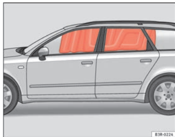
Fig. 26 Deployed curtain airbags
