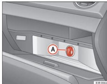
Fig. 138 Glove compartment with cool box open
