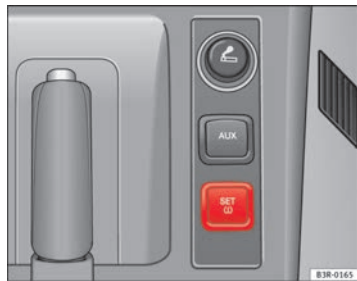
Fig. 188 Detailed view of the centre console: Button for the tyre pressure monitoring system
