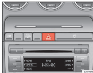
Fig. 92 Centre console: Switch for hazard warning lights
