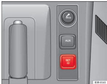
Fig. 173 Detailed view of the centre console: Button for the tyre pressure monitoring system
