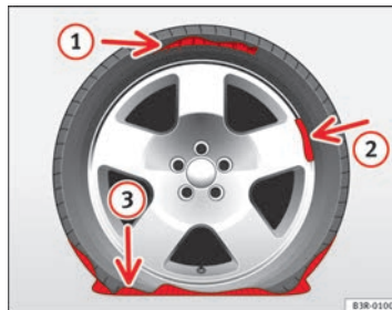
Fig. 183 The Tyre Mobility System is not suitable for repairing this type of damage to tyres.
