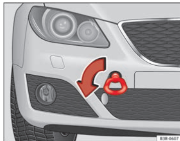
Fig. 227 Fitting the towing eye to front rear of the vehicle
