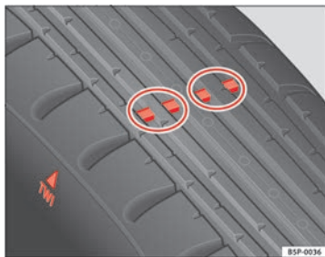
Fig. 174 Tyre tread wear indicators
