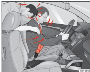
Fig. 9 The unbelted rear passenger is thrown forward violently, hitting the driver wearing a seat belt.
