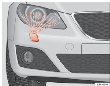
Fig. 102 Headlight with extended washer jet
