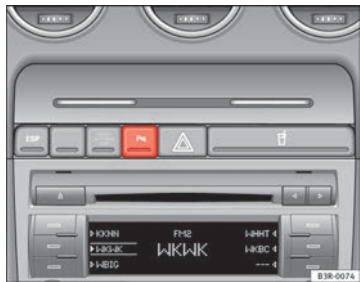
Fig. 139 Centre console: switch for parking aid
