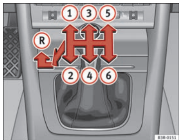
Fig. 142 Detailed view of the centre console: gear shift pattern of a 6-speed manual gearbox
