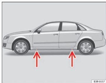
Fig. 180 Changing the wheel: Jack position points
