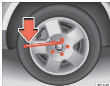
Fig. 179 Changing the wheel: Loosen the wheel bolts
