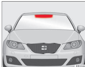
Fig. 162 Location of the electronic toll collection system
