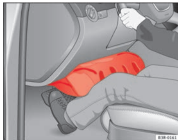
Fig. 22 Inflated airbags protect in a frontal collision.
