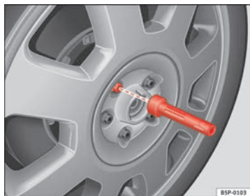
Fig. 182 Changing the wheel: Hexagonal socket in screwdriver handle to turn the wheel bolts
