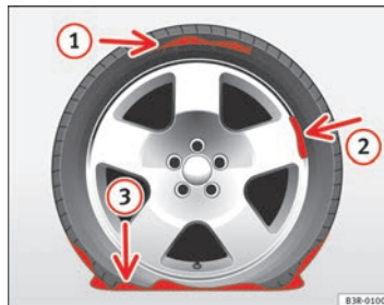
Fig. 184 The Tyre Mobility System is not suitable for repairing this type of damage to tyres.
