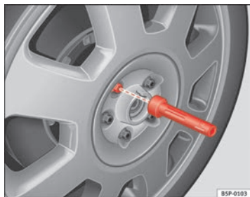
Fig. 186 Changing the wheel: Hexagonal socket in screwdriver handle to turn the wheel bolts
