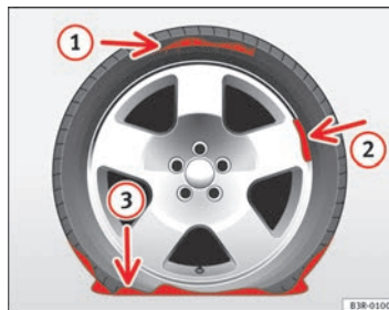
Fig. 188 The Tyre Mobility System is not suitable for repairing this type of damage to tyres.
