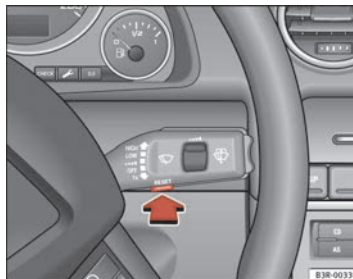
Fig. 61 Windscreen wiper lever: Menu selection button
