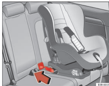
Fig. 33 The ISOFIX child seat anchorages slide along the fitted plastic guides until secured in the vehicle's ISOFIX anchorages
