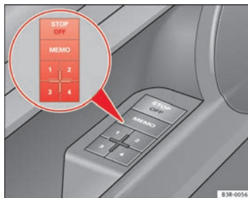
Fig. 110 Driver's door: Memory system
