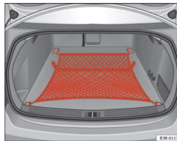
Fig. 117 Stretch net laid out
