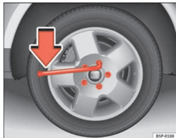
Fig. 183 Changing the wheel: Loosen the wheel bolts
