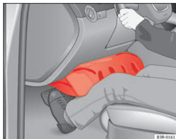
Fig. 22 Inflated airbags protect in a frontal collision.
