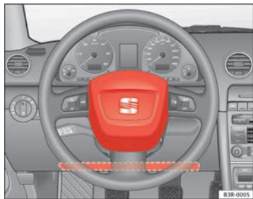
Fig. 17 Driver's Airbag in the steering wheel and knee airbag in the instrument panel
