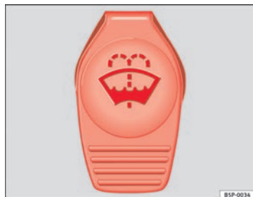
Fig. 173 In the engine compartment: Cap of windscreen washer fluid reservoir.
