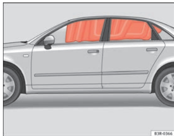
Fig. 26 Deployed curtain airbags
