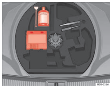
Fig. 181 Tyre Mobility System under floor panel in luggage compartment
