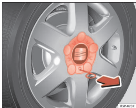
Fig. 131 Changing a wheel: Removing the wheel trim
