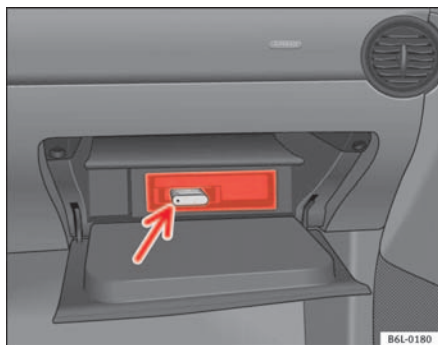
Fig. 84 iPod connection in the passenger side glove compartment
