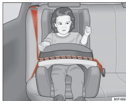
Fig. 27 A category 1 forward-facing child seat fitted on the rear seat.
