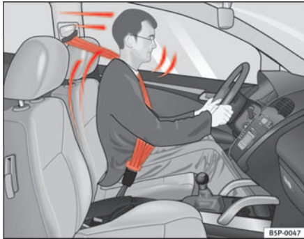
Fig. 10 Driver protected by the properly worn seat belt during a sudden braking manoeuvre.
