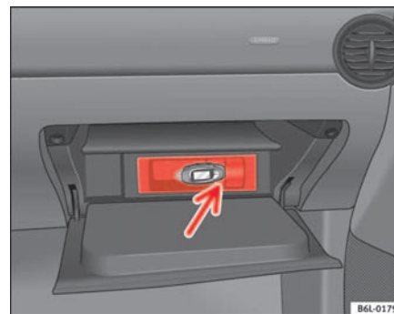
Fig. 85 USB* connection in the passenger side glove compartment
