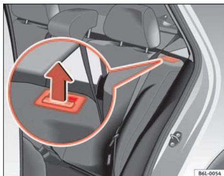
Fig. 74 Button for unlocking the rear backrest
