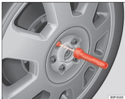
Fig. 136 Wheel change: Hexagon socket in screwdriver handle to turn the wheel bolts after they have been loosened
