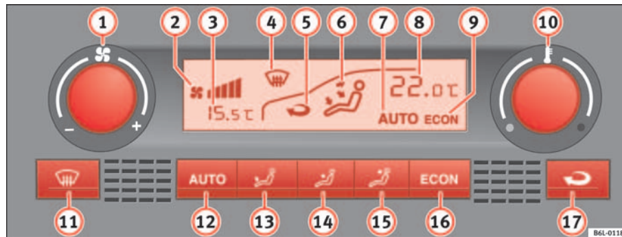
Fig. 91 On the instrument panel: Climatronic controls
