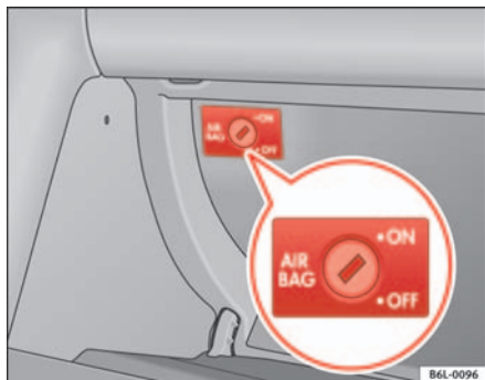
Fig. 24 In the glove box there is key switch for disabling and enabling the airbags on the front passenger side
