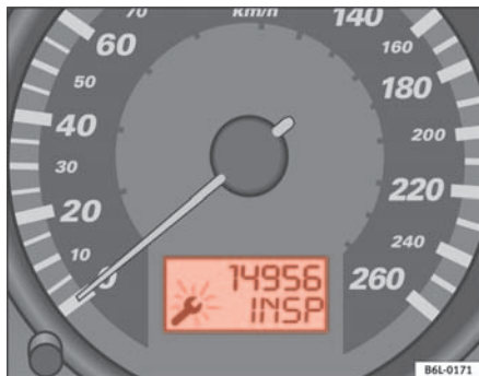
Fig. 38 Service interval display
