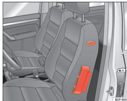
Fig. 20 Side airbag in driver seat
