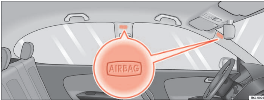
Fig. 22 Location of left curtain airbag
