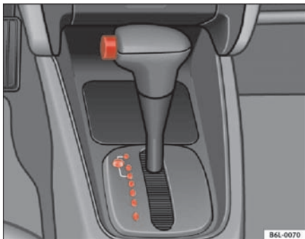
Fig. 98 Section of centre console: selector lever on cars with an automatic gearbox
