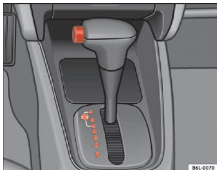
Fig. 97 Section of centre console: selector lever on cars with an automatic gearbox
