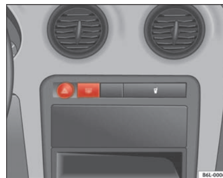
Fig. 58 Detail of the dash panel: Hazard warning light switch
