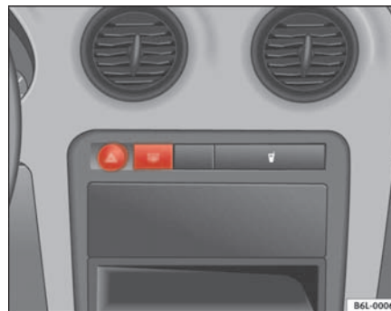
Fig. 57 Instrument panel: rear window heater switch ▶
