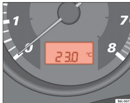
Fig. 37 Digital screen on the instrument panel: outside temperature display
