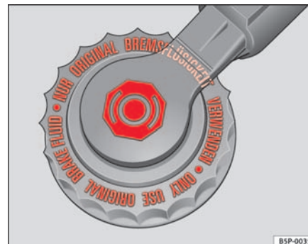
Fig. 128 In the engine compartment: Brake fluid reservoir cover
