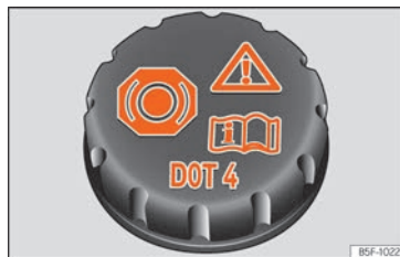
Fig. 207 Engine compartment: brake fluid reservoir cap.
