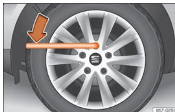
Fig. 222 Tyre change: slacken the wheel bolts.
