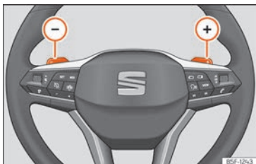
Fig. 103 Steering wheel: automatic gearbox levers
