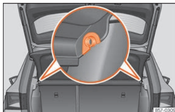
Fig. 166 In the boot: removing and installing the shelf.
