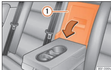
Fig. 176 On the rear seat backrest: opening the tailboard.
