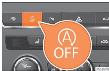
Fig. 99 Centre console: Start-Stop system button.
