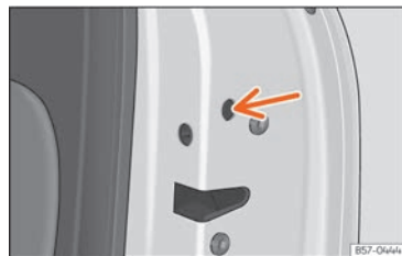
Fig. 57 Locking the door manually.
