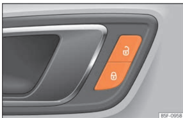
Fig. 54 On the driver's door: central locking button.
