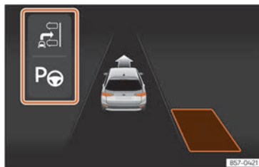
Fig. 139 On the instrument panel display: display of the assisted parking system with decreased visibility.
