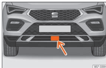
Fig. 108 On the front bumper: radar sensor.
