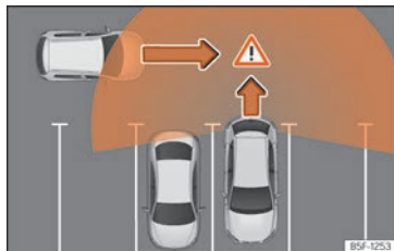
Fig. 150 Diagram of the parking assistant: detected area around the vehicle that is driving off.
