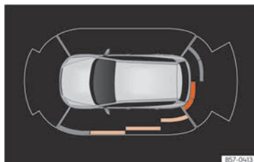
Fig. 136 Parking aid view on the Infotainment system display.
