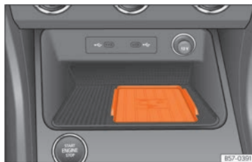
Fig. 164 Centre console: slot for mobile phone connection.
