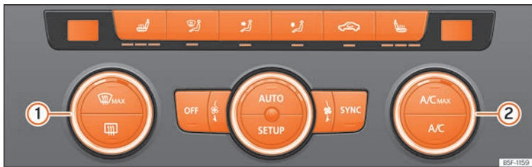
Fig. 92 In the centre console: Climatronic control panel.
