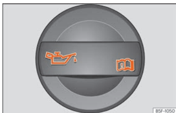
Fig. 212 Oil filler cap cover in the engine compartment.
