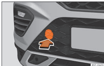
Fig. 193 Front bumper on right: remove the lid.
