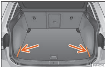
Fig. 167 In the boot: covers for storing the rear shelf.
