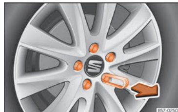
Fig. 220 Wheel: wheel bolts with caps.
