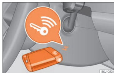
Fig. 98 On the right of the steering column: emergency start.
