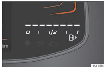
Fig. 5 Basic instrument cluster: fuel gauge.
