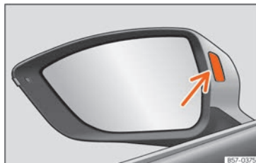
Fig. 127 Control lamp of the lane departure warning.
