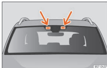
Fig. 95 Areas for placing electronic accessories
