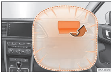
Fig. 28 Front passenger airbag located in dash panel.
