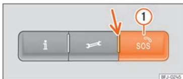
Fig. 44 On the roof console: controls for voice services
