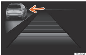
Fig. 151 On the instrument panel display: ACC active, vehicle detected in an outer lane.
