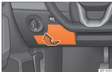
Fig. 48 On the driver's side dashboard: fuse box cover.
