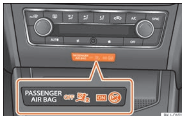
Fig. 17 Central part of the dashboard: control lamp for the deactivation of the front passenger front airbag.
