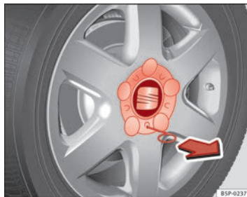
Fig. 177 Changing a wheel: Removing a hub cap
