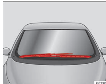
Fig. 170 Windscreen wipers in the service position
