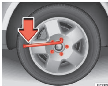
Fig. 178 Changing a wheel: loosen the wheel bolts
