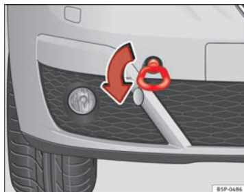
Fig. 206 The front right section of the vehicle: Fitting the front towline anchorage
