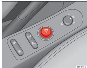
Fig. 118 The cigarette lighter is located in the electric socket on the front of the centre console
