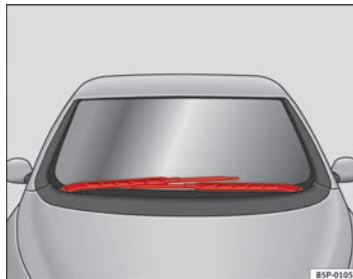
Fig. 171 Windscreen wipers in the service position
