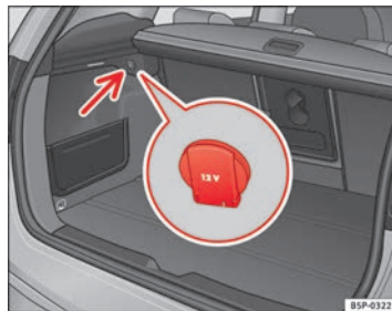
Fig. 120 Power socket in luggage compartment ►
