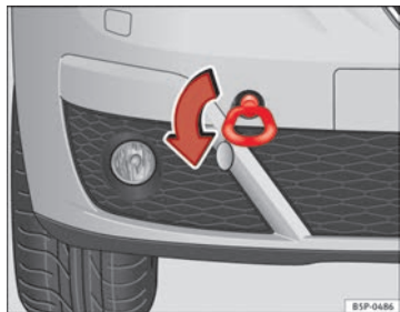
Fig. 207 The front right section of the vehicle: Fitting the front towing eye
