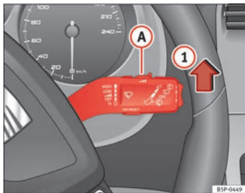
Fig. 88 Windscreen wiper lever
