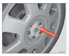
Fig. 176 Changing the wheel: Hexagonal socket in screwdriver handle to turn the wheel bolts
