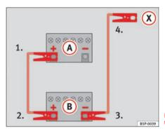
Fig. 199 How to connect the jump leads
