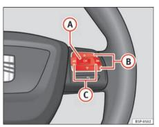
Fig. 44 Steering wheel controls: button A to confirm the menu selection and switch B to change the menu
