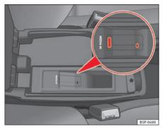
Fig. 122 Connection in central armrest compartment
