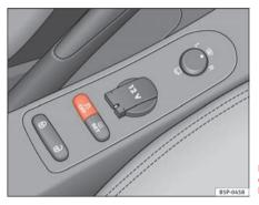
Fig. 137 Detail of the centre console: ESP button
