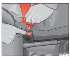
Fig. 16 Removing latch plate from buckle
