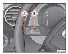
Fig. 149 Indicator and main beam headlight lever: switch and rocker switch for the cruise control
