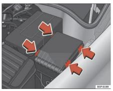
Fig. 179 Fuse box cover in engine compartment
