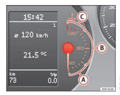
Fig. 35 Instrument panel: engine coolant temperature gauge
