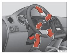
Fig. 135 Adjusting the steering wheel position
