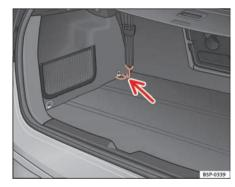
Fig. 126 Anchor rings for the separation net
