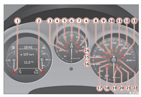
Fig. 48 Instrument panel with warning lamps. Some of the items of equipment listed here are fitted only on certain models/model years or are optional extras.
