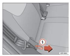
Fig. 98 Rear seat backrest angle adjustment
