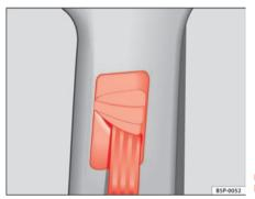
Fig. 17 Location of the belt height adjuster
