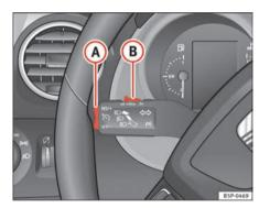
Fig. 152 Indicator and main beam headlight lever: switch and rocker switch for the cruise control
