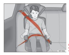
Fig. 30 Forward-facing child seat installed on rear seat.
