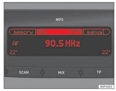
Fig. 133 Radio display with information about Climatronic
