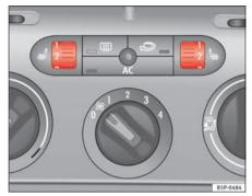
Fig. 95 Thumb wheel for the front seat heating
