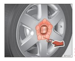
Fig. 171 Changing the wheel: Removing a hub
