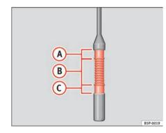
Fig. 159 Engine oil dipstick.
