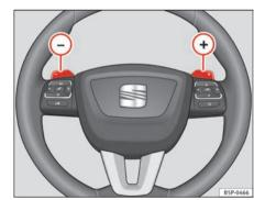
Fig. 146 Steering wheel with levers for automatic gearbox
