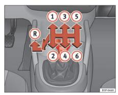
Fig. 140 Detail of the centre console: gear shift pattern of a 6-speed manual gearbox
