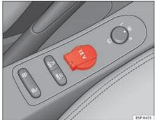
Fig. 118 Socket, centre console, front
