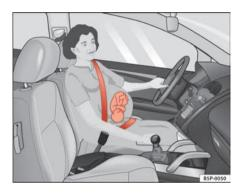
Fig. 15 Positioning seat belts during pregnancy
