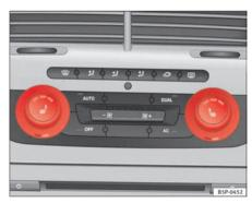
Fig. 96 Front seat heating with Climatronic
