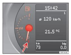
Fig. 34 Instrument panel: fuel gauge
