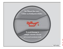
Fig. 160 In the engine compartment: Engine oil
