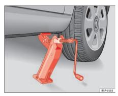
Fig. 174 Fitting the jack
