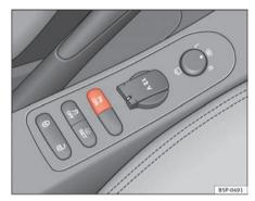
Fig. 148 Centre console: Switch for parking aid
