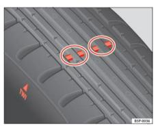
Fig. 168 Tyre tread wear indicators
