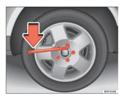
Fig. 172 Changing the wheel: loosen the wheel holts
