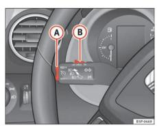
Fig. 153 Indicator and main beam headlight lever: switch and rocker switch for the cruise control
