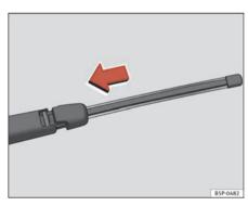
Fig. 166 Mount rear window wiper blade
