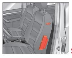
Fig. 22 Side airbag in driver seat
