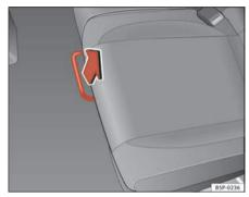
Fig. 97 For unlocking the rear seat
