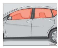
Fig. 25 Deployed curtain airbags
