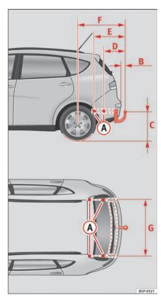
Fig. 154 Attachment points for towing bracket
