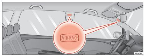
Fig. 24 Location of left curtain airbag
