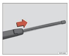
Fig. 165 Remove rear window wiper blade
