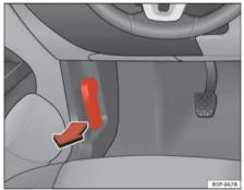
Fig. 156 Detail of footwell area on driver's side: lever for unlocking the bonnet.
