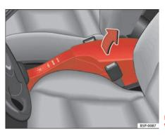
Fig. 102 Front armrest with stowage area
