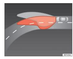
Fig. 75 Cornering lighting using self-directional headlights
