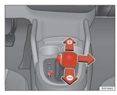
Fig. 145 Changing gear with Tiptronic
