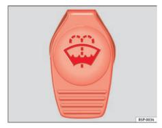
Fig. 162 In the engine compartment: Cap of windscreen washer fluid reservoir.
