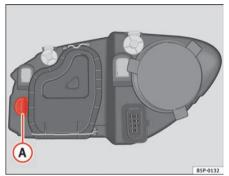
Fig. 181 Turn signal lamps
