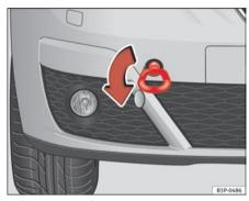
Fig. 200 The front right section of the vehicle: Fitting the front towing eye
