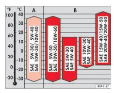
Fig. 158 Types of oil according to temperature
