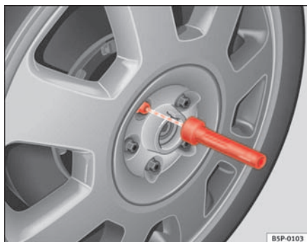
Fig. 175 Wheel change: Hexagon socket in screwdriver handle to turn the wheel bolts after they have been loosened
