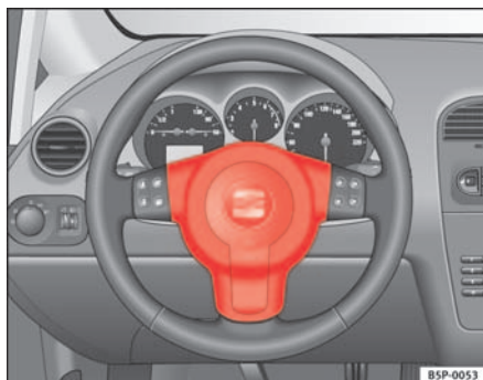
Fig. 18 Driver airbag located in steering wheel
