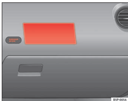
Fig. 19 Front passenger airbag located in dash panel
