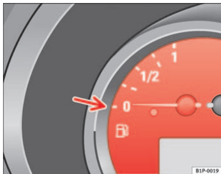
Fig. 34 Details of the instrument panel: Fuel gauge
