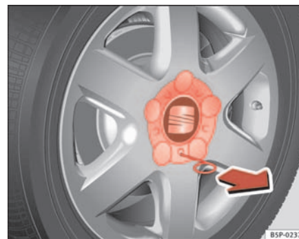
Fig. 171 Changing a wheel: Removing the wheel trim
