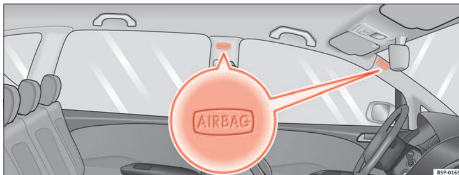
Fig. 24 Location of left curtain airbag
