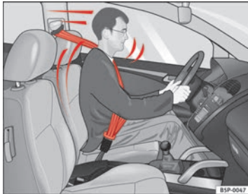
Fig. 11 A driver wearing the seat belt properly is secured by the belt in sharp braking
