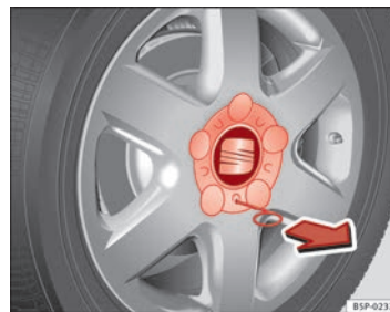
Fig. 169 Changing a wheel: Removing a hub cap
