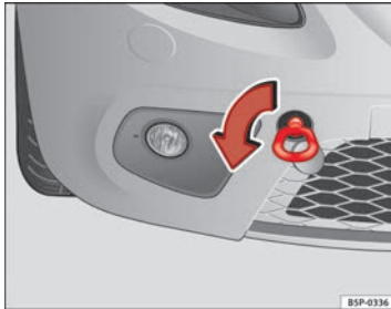
Fig. 198 The front right section of the vehicle: Fitting the front towline anchorage
