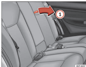
Fig. 108 Opening the rear drink holders
