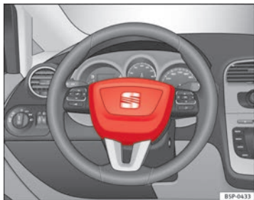
Fig. 18 Driver airbag located in steering wheel
