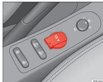
Fig. 116 Power socket in front centre console
