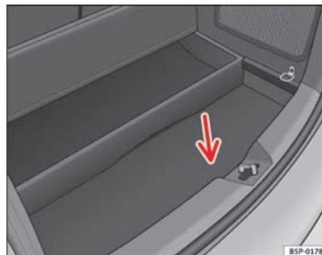
Fig. 168 Luggage compartment. Access to the spare wheel
