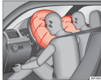
Fig. 20 Inflated front airbags
