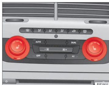
Fig. 94 Front seat heating with Climatronic
