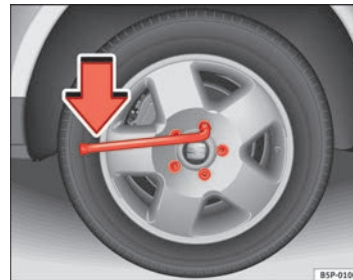
Fig. 170 Changing a wheel: loosen the wheel bolts
