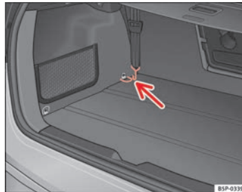
Fig. 124 Fastening rings for the separation net
