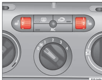
Fig. 93 Thumb wheel for the front seat heating
