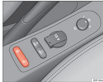
Fig. 57 Detailed view of the centre console: central lock button
