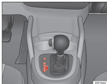
Fig. 141 Centre console: Selector lever for automatic gearbox / DSG automatic gearbox
