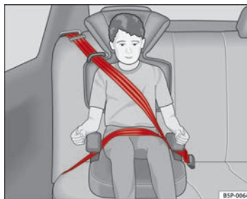
Fig. 30 Forward-facing child seat installed on rear seat
