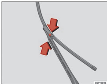
Fig. 163 Changing the front wiper blades
