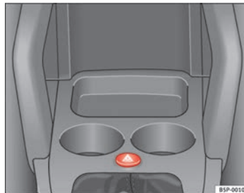
Fig. 74 Dash panel: switch for hazard warning lights
