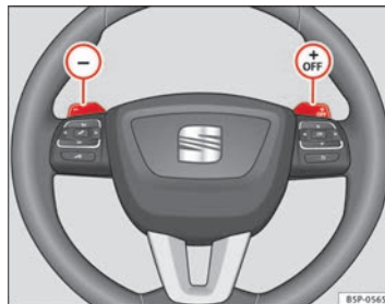
Fig. 146 Steering wheel with levers for automatic gearbox
