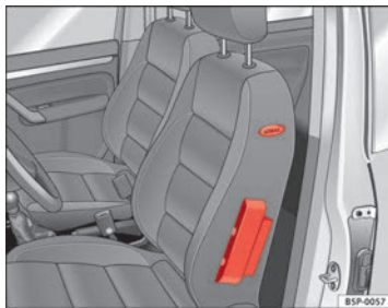
Fig. 22 Side airbag in driver seat
