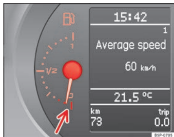
Fig. 35 Instrument panel: fuel gauge
