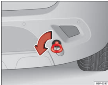
Fig. 199 Fitting the towline anchorage to the rear of the vehicle
