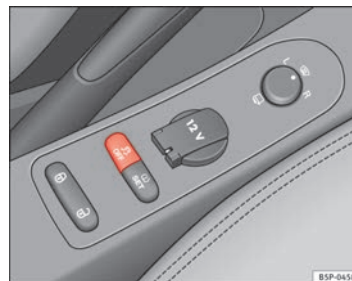
Fig. 135 Detailed view of the centre console: ESC switch.
