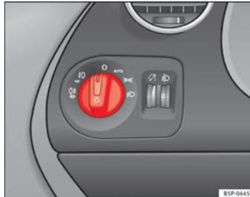
Fig. 70 Detailed view of the dash panel: lights, fog lights and rear fog light switch
