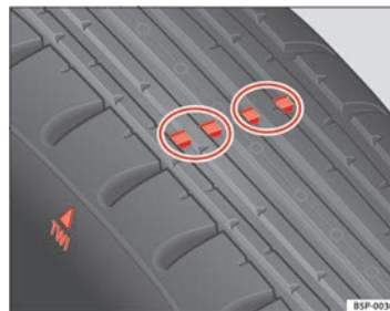
Fig. 166 Tyre tread wear indicators
