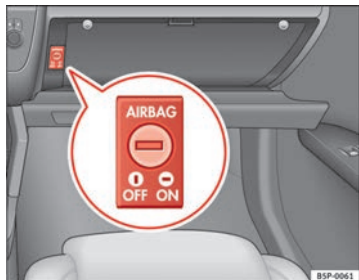
Fig. 26 In the glove compartment: switch for activating and deactivating the front passenger airbag
