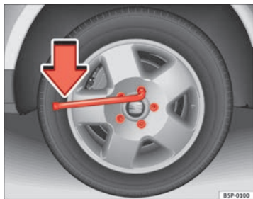
Fig. 171 Changing the wheel: loosen the wheel bolts
