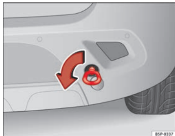
Fig. 200 Fitting the towing eye to the rear of the vehicle
