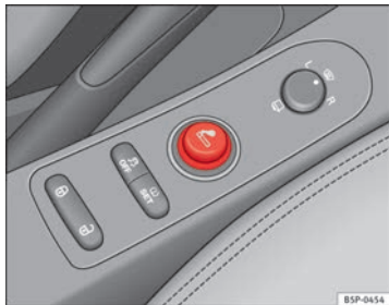
Fig. 116 The cigarette lighter is located in the electric socket on the front of the centre console
