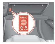
Fig. 26 In the glove compartment: switch for activating and deactivating the front passenger airbag
