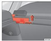
Fig. 123 Removing the rear shelf
