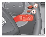
Fig. 87 Windscreen wiper and windscreen wash lever: rear window wiper
