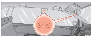
Fig. 24 Location of head airbags on the left side of the vehicle
