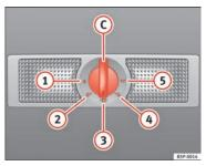
Fig. 81 Interior roof trim: rear interior lights and reading lights.
