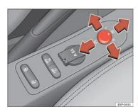
Fig. 89 Controls of exterior mirrors
