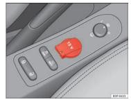
Fig. 117 Power socket in front centre console
