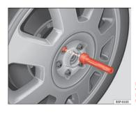
Fig. 173 Changing the wheel: Hexagonal socket in screwdriver handle to turn the wheel bolts
