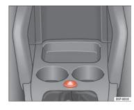
Fig. 75 Dash panel: switch for hazard warning liahts
