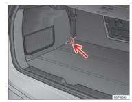
Fig. 125 Anchor rings for the separation net
