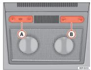
Fig. 79 Interior roof trim: front reading lights, type
