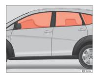
Fig. 25 Deployed curtain airbags
