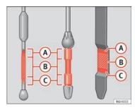
Fig. 157 Engine oil dipstick
