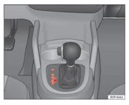
Fig. 140 Centre console: Selector lever for automatic gearbox / DSG automatic gearbox
