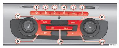
Fig. 130 On the dash panel: 2C Climatronic controls
