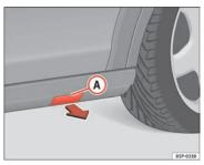
Fig. 172 Plastic sill panel trim with jack allotment cover
