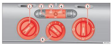
Fig. 127 On the dash panel: Climatic controls
