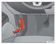
Fig. 155 Detail of footwell area on driver side: lever for unlocking the bonnet.
