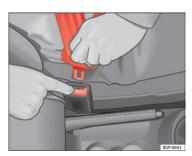
Fig. 16 Removing latch plate from buckle
