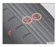
Fig. 165 Tyre tread wear indicators
