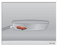
Fig. 194 Removing sun visor light
