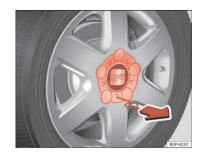
Fig. 168 Changing the wheel: Removing a hub cap
