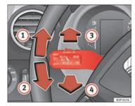
Fig. 76 Turn signal and main beam headlight lever
