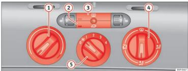
Fig. 126 Heating controls on the dash panel
