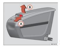
Fig. 113 Mobile storage compartment. Opening
