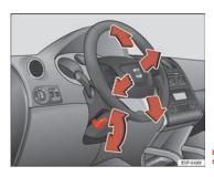
Fig. 134 Adjusting the steering wheel position
