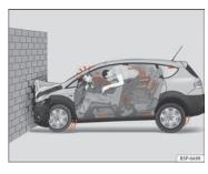
Fig. 8 The vehicle hits the wall: the occupants are not wearing seat belts
