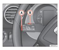
Fig. 148 Turn signal and main beam headlight lever: switch and rocker switch for the cruise control
