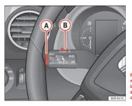
Fig. 147 Turn signal and main beam headlight lever: switch and rocker switch for the cruise control
