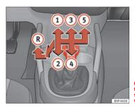
Fig. 138 Detailed view of the centre console: gear shift pattern of a 5-speed manual gearbox
