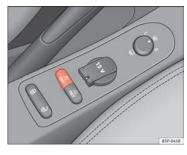
Fig. 136 Detailed view of the centre console: ESP button
