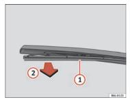
Fig. 163 Changing the rear window wiper blade
