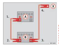
Fig. 196 Diagram for connecting jump leads if the vehicle providing assistance the current is not fitted with the Start-Stop system: flat battery (A) and battery providing current (B).
