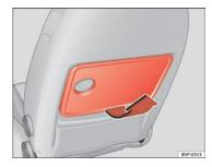
Fig. 103 Folding tray on the front left seat
