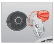
Fig. 154 Tank flap open
