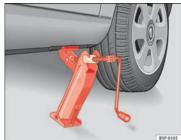
Fig. 171 Fitting the jack
