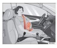
Fig. 15 Positioning seat belts during pregnancy
