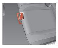
Fig. 96 For unlocking the rear seat
