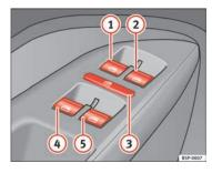
Fig. 67 Detail of the driver door: controls for the front and rear windows
