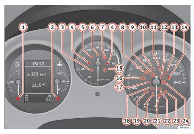
Fig. 49 Instrument panel indicator and warning lamps. Some of the items of equipment listed here are fitted only on certain model versions or are optional extras.
