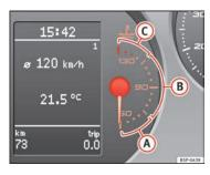
Fig. 36 Instrument panel: engine coolant temperature gauge
