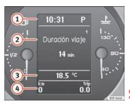
Fig. 38 Digital instrument panel display
