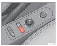
Fig. 50 Centre console: tyre monitor system button
