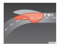
Fig. 74 Cornering lighting using adaptive headlights
