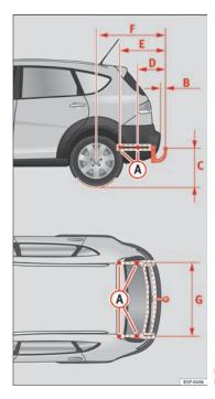
Fig. 153 Attachment points for towing bracket
