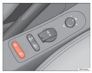
Fig. 57 Detailed view of the centre console: central locking button
