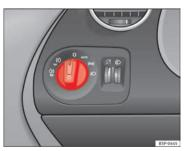
Fig. 71 Detailed view of the dash panel: lights, fog lights and rear fog light switch
