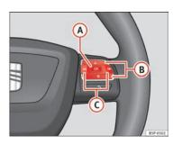
Fig. 45 Steering wheel controls: button A to confirm the menu selection and switch B to change the menu
