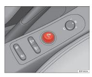
Fig. 116 The cigarette lighter is located in the power socket on the front of the centre console
