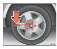
Fig. 169 Changing the wheel: loosen the wheel holts
