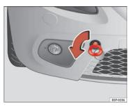
Fig. 198 The front right section of the vehicle: Fitting the front towing eye
