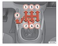
Fig. 139 Detailed view of the centre console: gear shift pattern of a 6-speed manual gearbox
