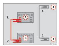
Fig. 197 Diagram for connecting jump leads if the vehicle providing assistance is fitted with the Start-Stop system: flat battery (A) and battery providing current
