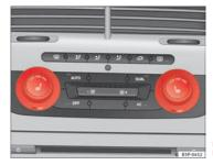
Fig. 95 Front seat heating with Climatronic
