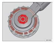
Fig. 164 In the engine compartment: Brake fluid reservoir cover
