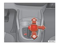
Fig. 144 Changing gear with tiptronic
