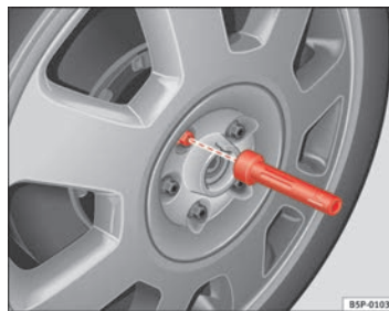
Fig. 175 Changing the wheel: Hexagonal socket in screwdriver handle to turn the wheel bolts
