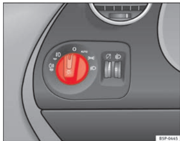
Fig. 72 Detailed view of instrument panel: lights, fog light and rear fog light control
