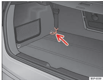
Fig. 126 Anchor rings for the separation net
