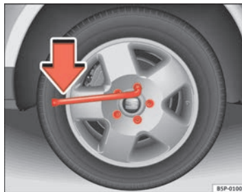
Fig. 171 Changing the wheel: loosen the wheel bolts
