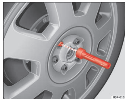
Fig. 181 Changing the wheel: hexagonal socket in screwdriver handle to turn the wheel bolts after they have been loosened
