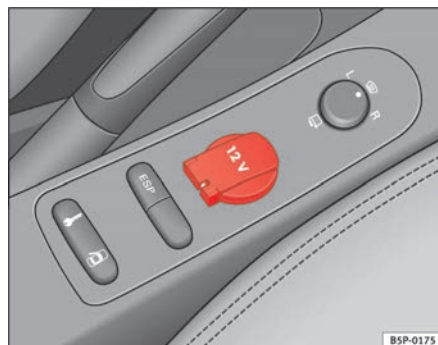
Fig. 118 Socket, centre console, front
