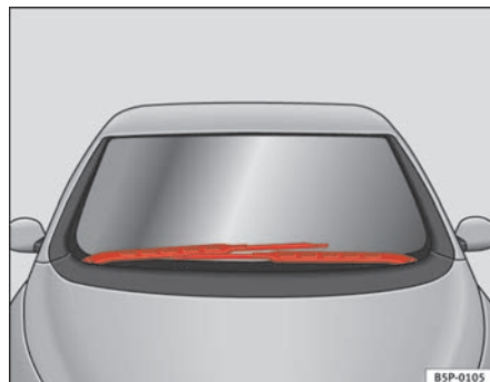
Fig. 169 Windscreen wipers in the service position
