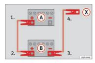
Fig. 208 Diagram of connections for vehicles without Start-Stop system.
