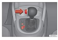
Fig. 142 Centre console: Automatic gearbox selector lever
