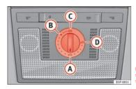
Fig. 66 Roof lining description: sliding/tilting sunroof rotary knob
