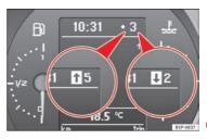
Fig. 40 Gear display.
