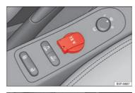
Fig. 111 Power socket, centre console, front
