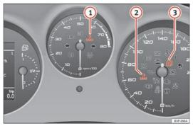
Fig. 47 Instrument panel control and warning lamps in vehicles with LPG
