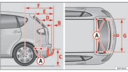
Fig. 151 Attachment points for towing bracket.
