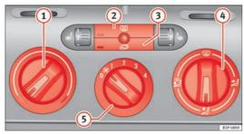
Fig. 125 Heating controls on the dash panel.
