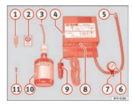
Fig. 178 Standard representation: contents of the anti-puncture kit.
