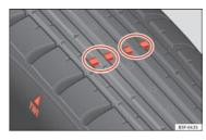
Fig. 168 Tyre tread wear indicators.
