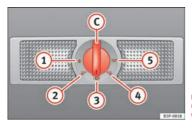
Fig. 76 Interior roof trim: rear interior lights and reading lights.
