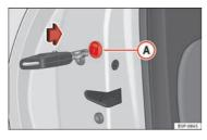
Fig. 56 Locking the doors manually.
