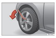
Fig. 173 Changing a wheel: loosen the wheel holts
