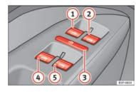
Fig. 65 Detail of the driver door: controls for the front and rear windows
