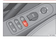
Fig. 136 Centre console: gas system control switch.
