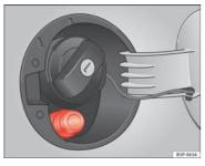
Fig. 156 Fuel tank flap open with EURO-type connector.
