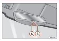
Fig. 83 Automatic antidazzle interior rear vision mirror.
