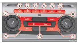
Fig. 131 On the dash panel: 2C Climatronic controls.
