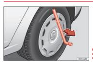
Fig. 172 Changing a wheel: remove the wheel cover.
