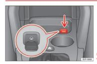
Fig. 113 Auxiliary audio connection
