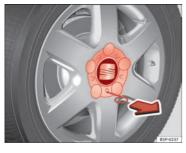
Fig. 171 Changing a wheel: removing a hub
