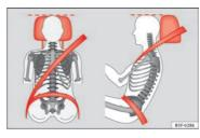
Fig. 3 Correctly adjusted head restraint viewed from the front and the side.
