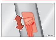
Fig. 15 Location of the belt height adjuster.
