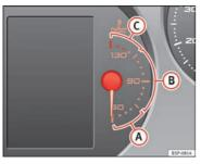
Fig. 37 Instrument panel: engine coolant temperature gauge.
