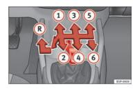
Fig. 139 Detailed view of the centre console: gear shift pattern of a 5 or 6speed manual gearbox
