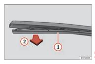
Fig. 166 Changing the rear window wiper blade.
