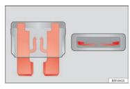
Fig. 181 Image of a blown fuse
