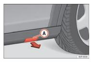
Fig. 176 Plastic sill panel trim with jack allotment cover
