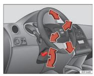
Fig. 132 Adjusting the steering wheel position
